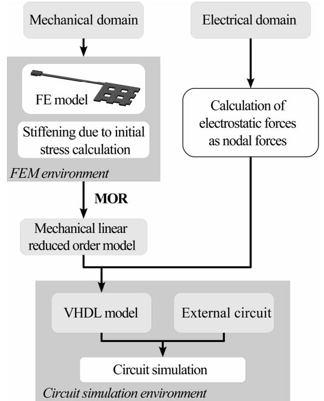
Fig 1::Block diagram of the simulation approach for RF MEMS switch devices.
