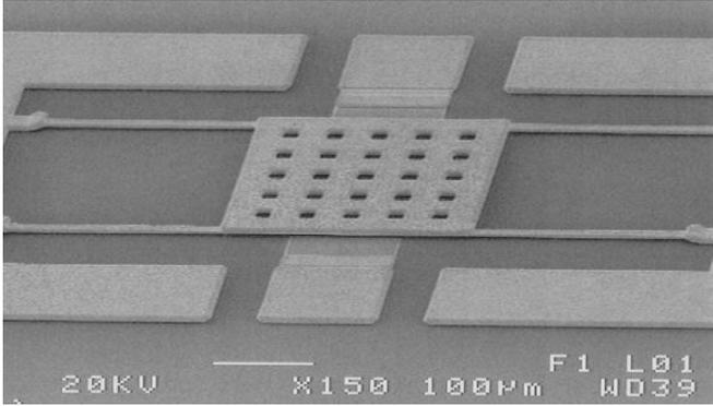
Fig. 2: SEM picture of the capacitive RF switch used in measurements and simulations.
