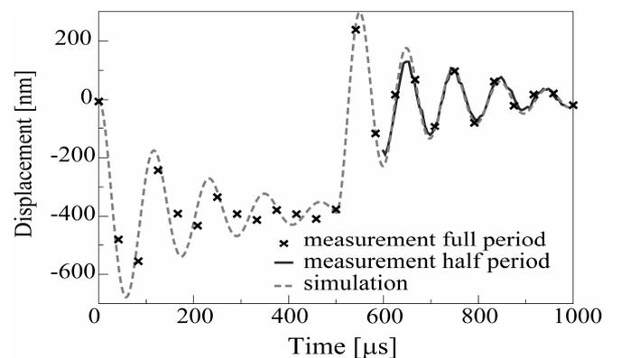
Fig. 3: Switch response to a square wave actuation voltage. Circuit simulation results are compared with two sets of experimental data.
