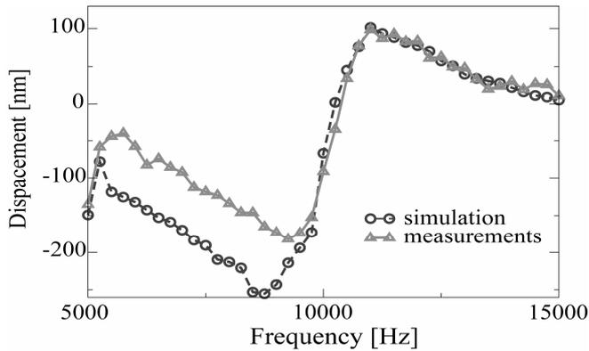
Fig 4: Circuit simulation results and measurements of the large signal response of the switch to a sinusoidal actuation voltage.
