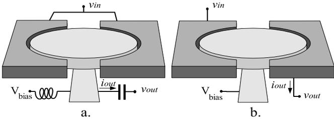
Fig. 1. Measurement setup of a disk resonator in a one-port (a.) and two-port (b.) configuration.
