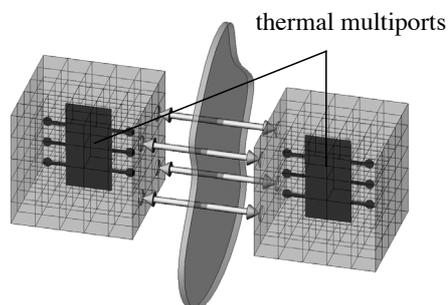
**Fig. 7** Continuous thermal flux through the shared interface of two FE models. The goal is to model the “FE cubes” as thermal multiports i. e. to lump a flux.
