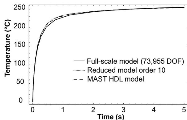
**Fig. 8** Solution of the full-scale system (73.955 DOF) and of the reduced order 10 system in a central hotplate node of gas sensor device.
