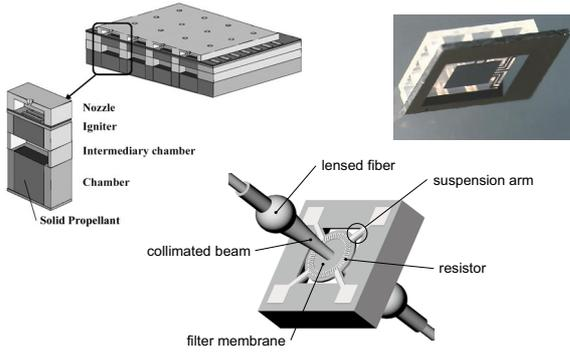
**Fig. 2** MEMS case studies: microthruster (top left), gas sensor (top right), optical filter (bottom).
