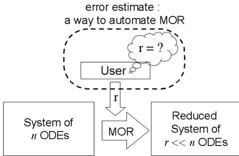
**Fig. 5** Compact model extraction. Eliminating the need for user iteration makes the process fully automatic.
