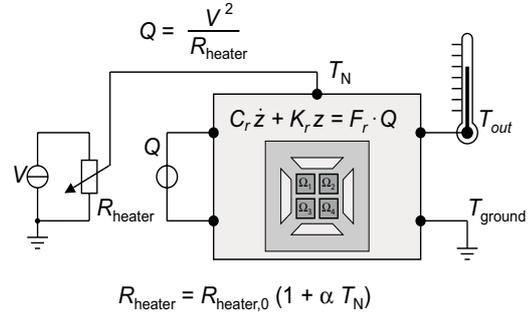
**Fig. 3** HDL model structure containing back coupled temperature dependant heater
