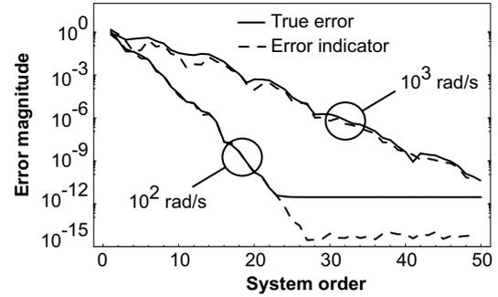
**Fig. 6** Convergence of relative error between the two successive reduced models for the microthruster.
