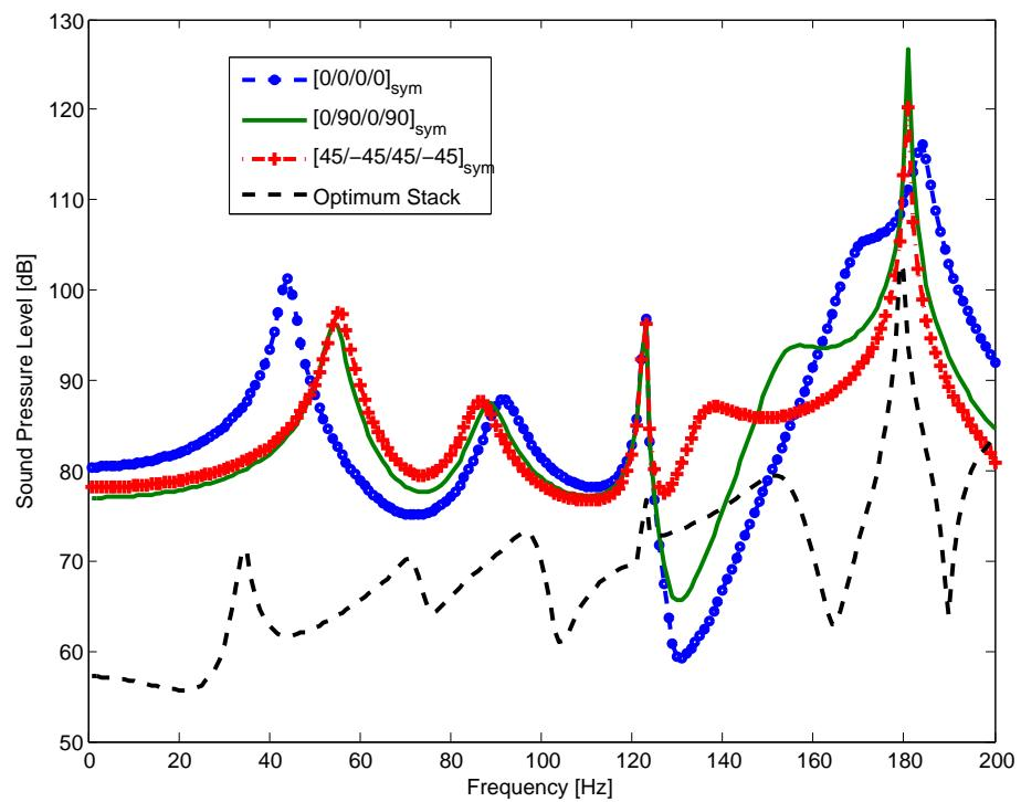
Figure 6.15.: A comparison of Arnoldi predicted fluid pressure for composite (PP-Glass) stacking sequences:  $[0/0/0/0]_{sym}$ ,  $[0/90/0/90]_{sym}$ ,  $[30/-30/30/-30]_{sym}$  and optimum stacking sequence  $[166/6/59/18/52/31/17/59]$  obtained by LHS/MADS optimization.
