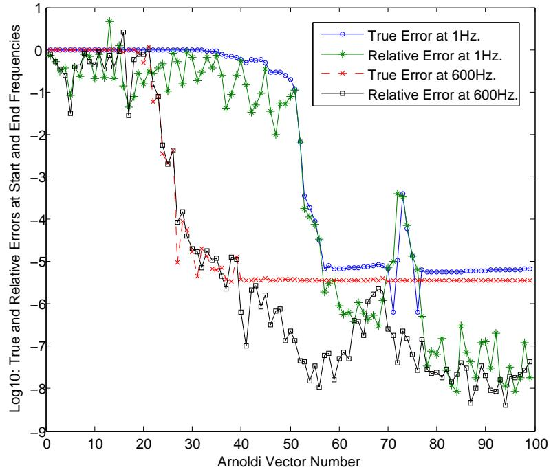
Figure 5.106.: Convergence pattern for moment-matching Arnoldi (OSA) projection at 1Hz and 600Hz for  $\zeta=0.05$ .
