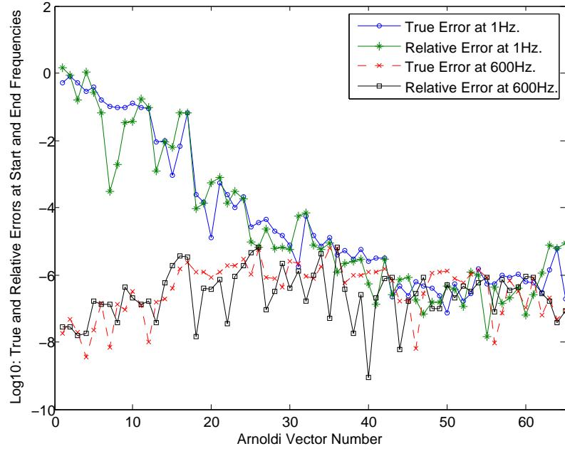
Figure 5.112.: Convergence plot for fluid node at the center of the cylindrical cavity with  $\beta_j^m=5.0\text{E-}05$ .
