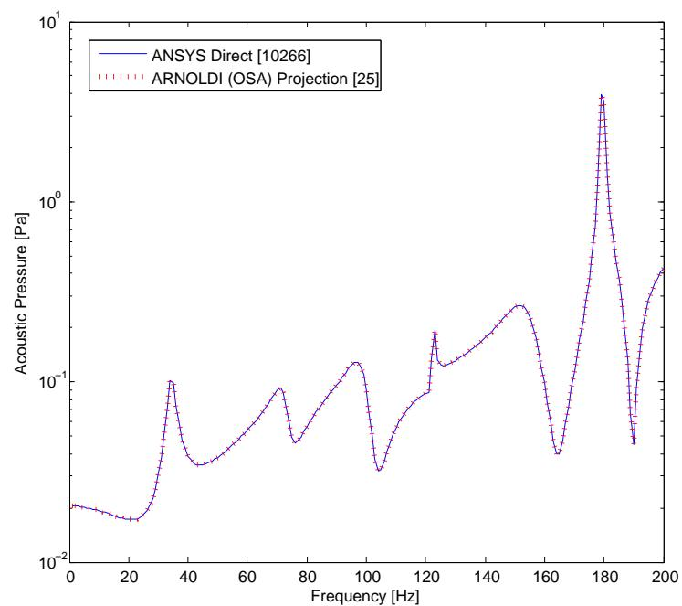
Figure D.3.: A comparison of noise transfer function obtained by ANSYS direct and One-sided Arnoldi (OSA) projection for optimized 8 layer stacking sequence (with material PP-Glass Fiber composite).
