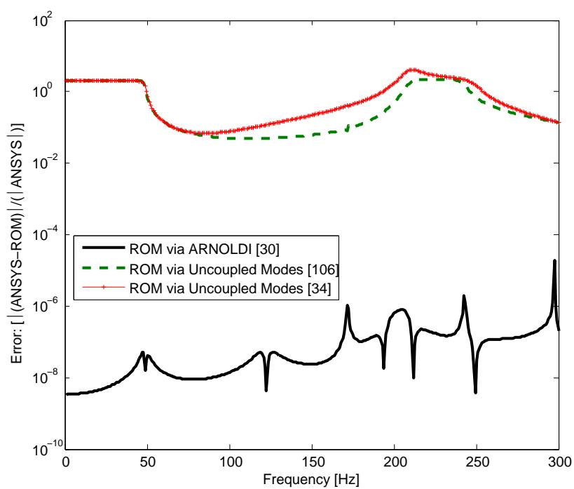
Figure 5.56.: A comparison of error quantities for noise transfer function for fluid node at  $(0.5\text{m}, 0.5\text{m}, 0.5\text{m})$  obtained using Arnoldi projection, Uncoupled modes approach (Full) and Truncated uncoupled modal approach for  $\zeta=0.03$ .
