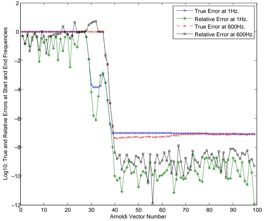
Figure 5.70.: Convergence pattern for moment-matching Arnoldi (OSA) projection at 1Hz and 600Hz for  $\zeta=0.05$ .
