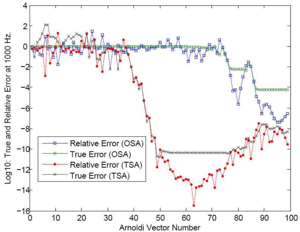
Figure 5.14.: Test Case No. 1: Convergence Plot: OSA, TSA convergence at 1000Hz.
