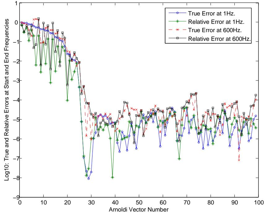
Figure 5.82.: Convergence pattern for moment-matching Arnoldi (TS-SOAR) projection at 1Hz and 600Hz for  $\beta_j^m=4.0\text{E-}05$ .
