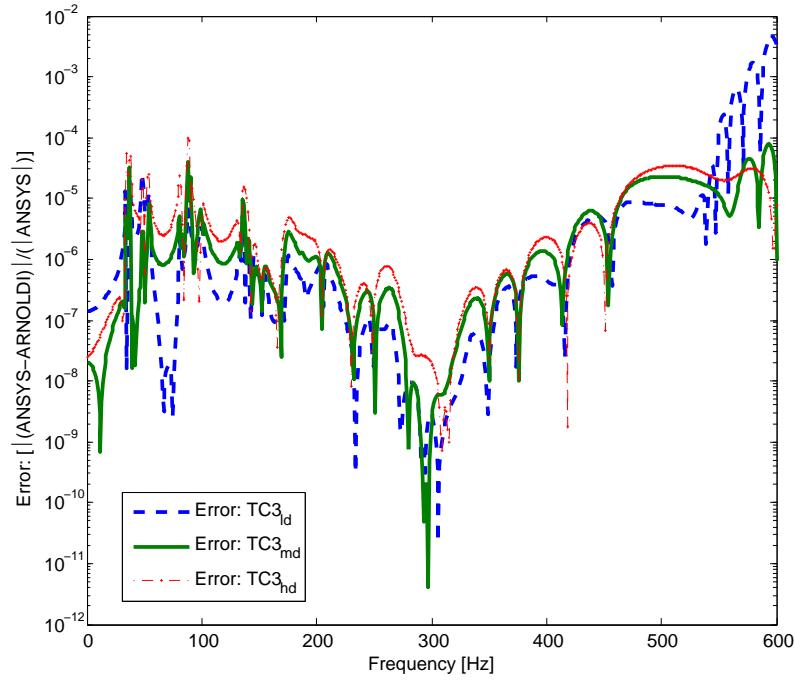
Figure 5.77.: Error plot for Predicted Driving Point Displacement Transfer Function (Receptance) at  $(0.039\text{m}, 0.14\text{m}, 0.078\text{m})$  for TS-SOAR projection for damping values:  $\beta_j^m = 2.0\text{E-}05$  [ $\text{TC3}_{ld}$ ],  $\beta_j^m = 4.0\text{E-}05$  [ $\text{TC3}_{md}$ ],  $\beta_j^m = 6.0\text{E-}05$  [ $\text{TC3}_{hd}$ ].
