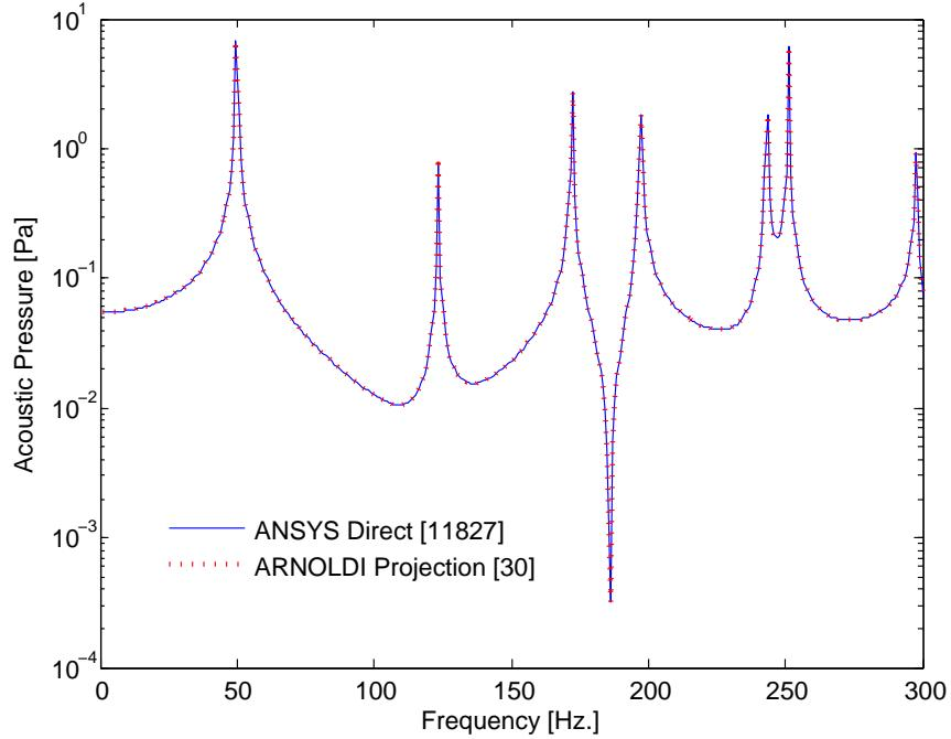
Figure 5.28.: Test Case No. 2: Predicted Noise Transfer Function using direct and moment-matching Arnoldi projection for fluid node at (0.35m,0.65m,0.3m).
