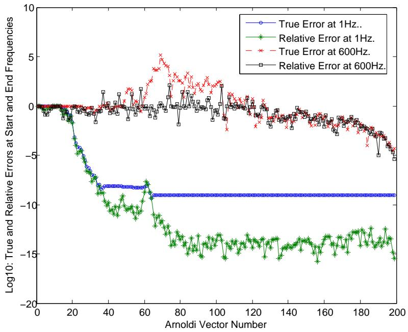
Figure 5.115.: Convergence plot for moment-matching Linearized Arnoldi (OSA) for fluid node at the center of the cylinder with  $\beta_j^m=7.0\text{E-}05$ .
