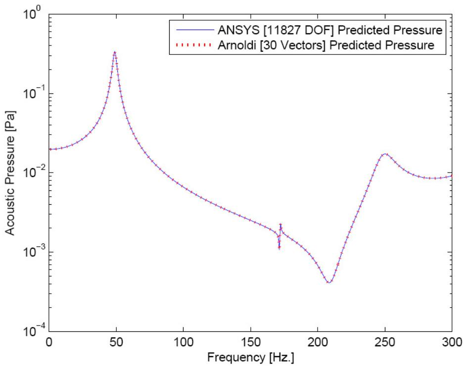
Figure 5.40.: ANSYS and moment matching Arnoldi projection predicted fluid pressure at  $(0.5\text{m}, 0.5\text{m}, 0.5\text{m})$  for  $\zeta=0.03$ .
