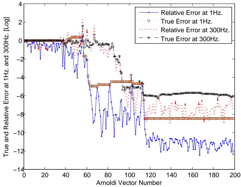
Figure 5.123.: Test Case No. 5: Convergence pattern for Arnoldi vectors ( $f_{exp}^2=150\text{Hz}$ ) at approximately 1Hz and 300Hz.
