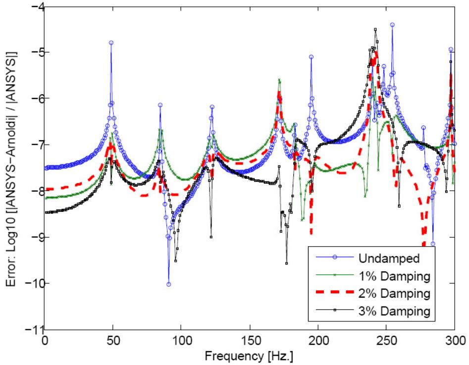
Figure 5.42.: Local Error plot for fluid node at  $(0.75\text{m}, 0.75\text{m}, 0.25\text{m})$  for  $\zeta=0, 0.01, 0.02, 0.03$ .
