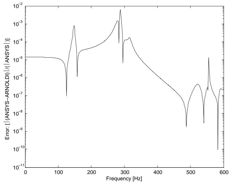
Figure 5.88.: Error plot for ANSYS and TSA predicted Noise Transfer Functions (NTF) for fluid node at (0.135m,0.07m,0.175m).
