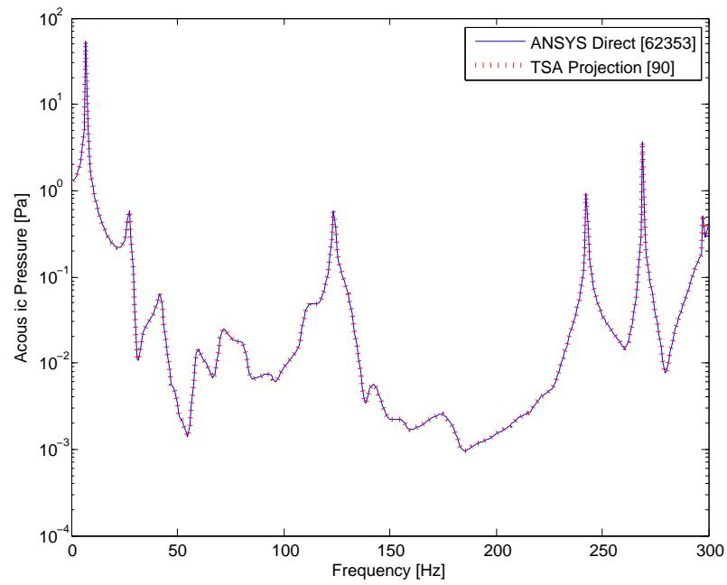
Figure C.4.: Test Case No. 6: ANSYS and TSA projection predicted Noise Transfer Function at fluid node (0.9m,0.5m,0.08m) for model TC6<sub>BM</sub>.
