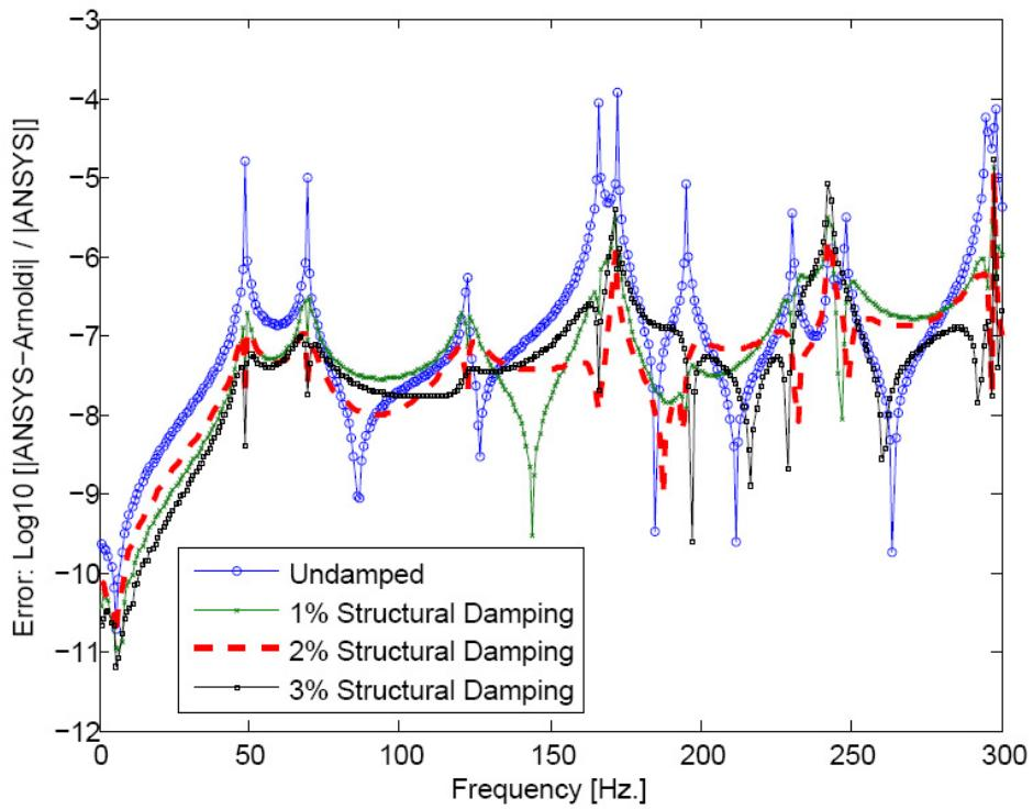
Figure 5.41.: Local Error plot for structural node at  $(0.25\text{m}, 1\text{m}, 0.65\text{m})$  for  $\zeta=0, 0.01, 0.02, 0.03$ .
