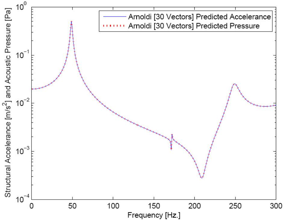
Figure 5.36.: Moment matching Arnoldi projection predicted vibro-acoustic reciprocity transfer functions for structural node at  $(0.25\text{m}, 1.0\text{m}, 0.65\text{m})$  and fluid node at  $(0.5\text{m}, 0.5\text{m}, 0.5\text{m})$  for  $\zeta=0.02$ .
