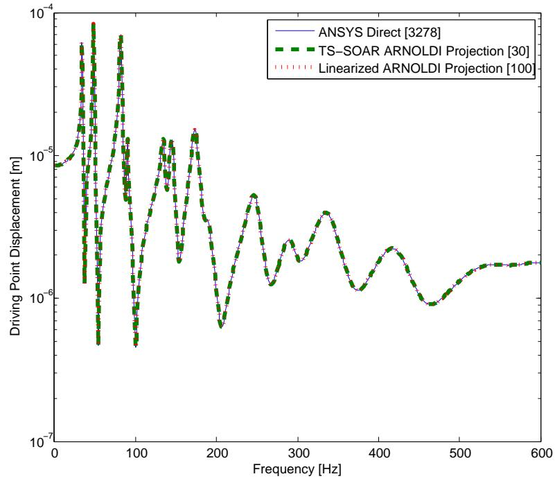
Figure 5.75.: Predicted Driving Point Displacement Transfer Function (Receptance) using direct and moment-matching Linearized Arnoldi and TS-SOAR projection for structural node at (0.039m,0.14m,0.078m) for  $\beta_j^m=4.0\text{E-}05$ .
