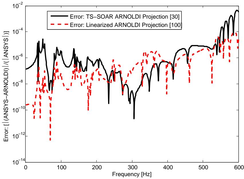
Figure 5.78.: Error plot for Predicted Driving Point Displacement Transfer Function (Receptance) at  $(0.039\text{m}, 0.14\text{m}, 0.078\text{m})$  for Linearized ARNOLDI and TS-SOAR projections with damping value  $\beta_j^m = 2.0\text{E-}05$  [ $\text{TC3}_{ld}$ ].
