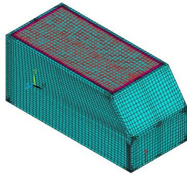
Figure 5.128.: Test Case No. 6: Coupled Structural-Acoustic model.
