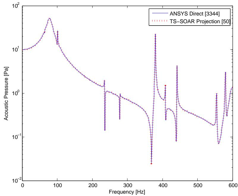
Figure 5.89.: Predicted Noise Transfer Function (NTF) using direct and moment-matching TSA projection for fluid node at (0.135m,0.07m,0.175m) for the air filled, free-free plate model.
