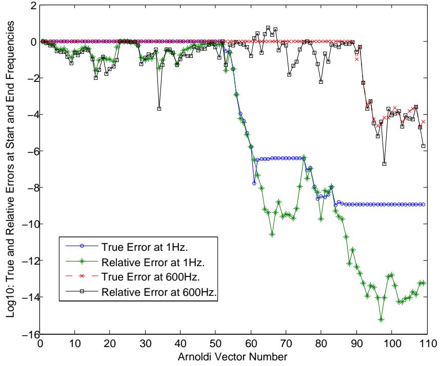
Figure 5.85.: Convergence pattern for moment-matching Linearized Arnoldi projection at 1Hz and 600Hz for  $\beta_j^m=4.0\text{E-}05$ .
