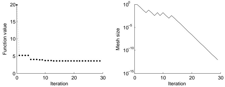
Figure 6.6.: Change in RMS objective function value (*left*) and mesh size (*right*) during optimization with initial 100 samples from LHS and starting stacking sequence  $[0/0]_{sym}$
