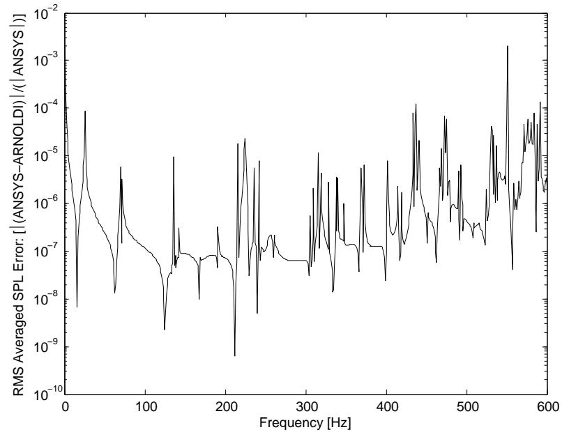
Figure 5.99.: Local RMS Averaged Error Plot utilizing 21 fluid pressure outputs [TC4<sub>FF</sub>].
