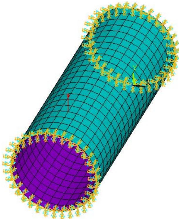
Figure 5.91.: Test Case No. 4: Clamped Cylindrical cavity (air filled) system - Structural Finite Element model. Excitation location: (0.039m,0.14m,0.078m); Measurement location(s): 21 fluid grid points along the central axis of the cylinder.
