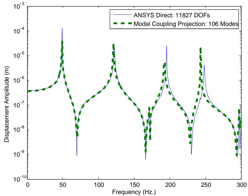
Figure 5.51.: ANSYS direct and uncoupled modes (fluid+structure) projection predicted driving point displacement transfer functions for structural node at (0.25m,1m,0.65m) for  $\zeta=0$ .
