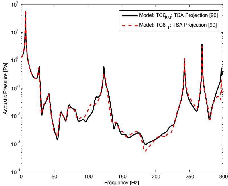
Figure 5.129.: Test Case No. 6: Predicted Noise Transfer Function using direct and moment-matching Two Sided Arnoldi projection for fluid node at (0.9m,0.5m,0.08m) for adhesively bonded coupled models [TC6<sub>BM</sub>] and [TC6<sub>TT</sub>].
