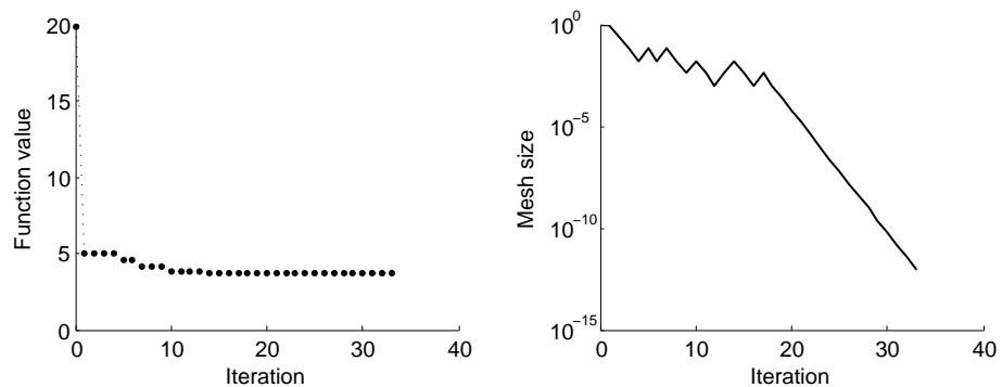
Figure 6.5.: Change in RMS objective function value (*left*) and mesh size (*right*) during optimization with initial 50 samples from LHS and starting stacking sequence  $[0/0]_{sym}$
