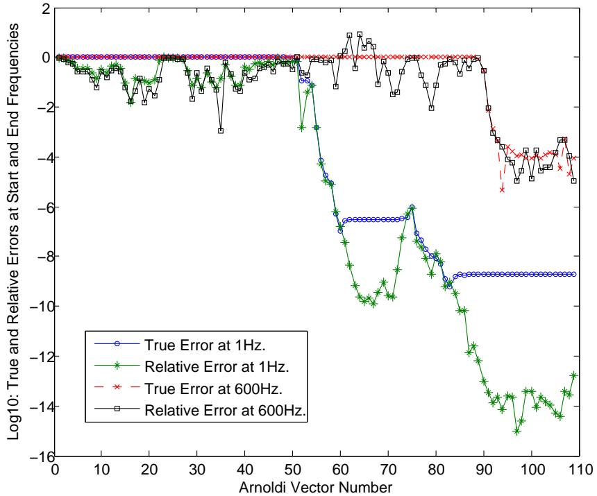
Figure 5.84.: Convergence pattern for moment-matching Linearized Arnoldi projection at 1Hz and 600Hz for  $\beta_j^m=2.0\text{E-}05$ .
