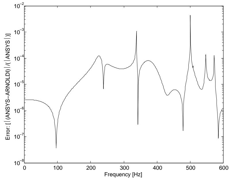
Figure 5.111.: Local Error Plot for fluid node at the center of the cylindrical cavity with  $\beta_j^m=5.0\text{E-}05$ .
