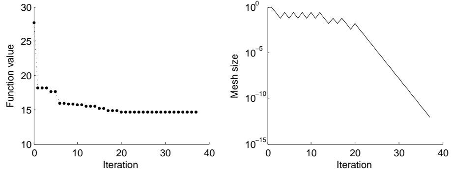
Figure 6.12.: Change in RMS objective function value (*left*) and mesh size (*right*) during optimization with initial 50 samples from LHS and with a starting stacking sequence  $[0/0/0/0]_{sym}$  for PP-Glass fiber composite.
