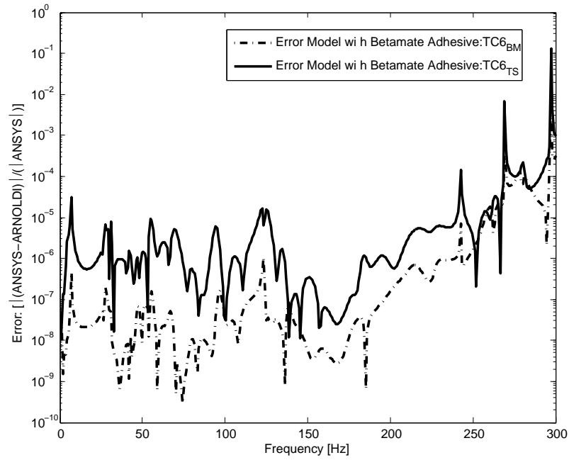
Figure 5.130.: Test Case No. 6: Noise Transfer Function error plot for fluid node at  $(0.9\text{m}, 0.5\text{m}, 0.08\text{m})$  for adhesively bonded coupled models  $[\text{TC6}_{\text{BM}}]$  and  $[\text{TC6}_{\text{TT}}]$ .
