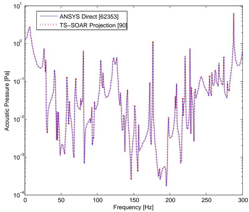
Figure 5.133.: Test Case No. 6: Predicted Noise Transfer Function using direct and moment-matching Two Sided Second order Arnoldi (TS-SOAR) projection for fluid node at (0.9m,0.5m,0.08m) with constant acoustic damping [TC6<sub>Tac</sub>].
