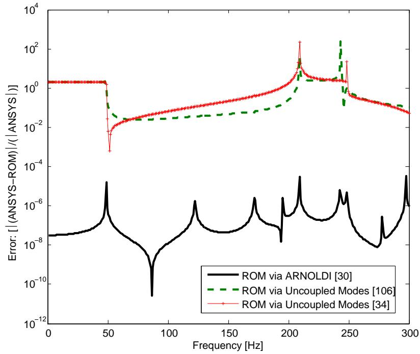
Figure 5.54.: A comparison of error quantities for noise transfer function for fluid node at  $(0.5\text{m}, 0.5\text{m}, 0.5\text{m})$  obtained using Arnoldi projection, Uncoupled modes approach (Full) and Truncated uncoupled modal approach for  $\zeta=0$ .
