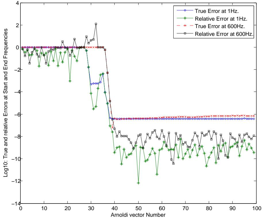
Figure 5.68.: Convergence pattern for moment-matching Arnoldi (OSA) projection at 1Hz and 600Hz for  $\zeta=0.03$ .
