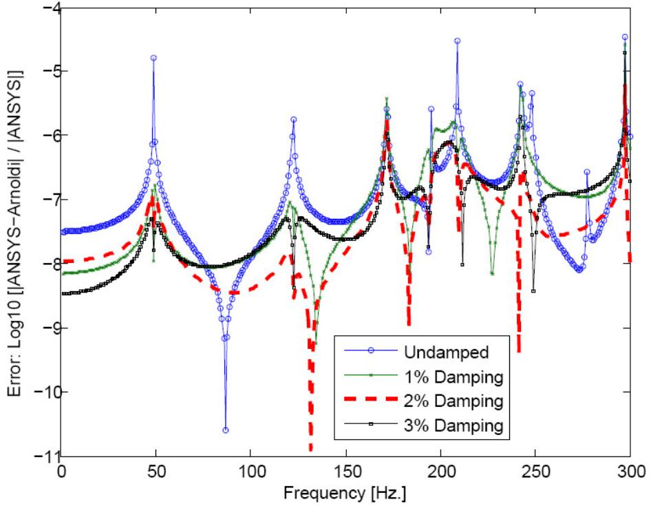
Figure 5.44.: Local Error plot for fluid node at  $(0.5\text{m}, 0.5\text{m}, 0.5\text{m})$  for  $\zeta=0, 0.01, 0.02, 0.03$ .
