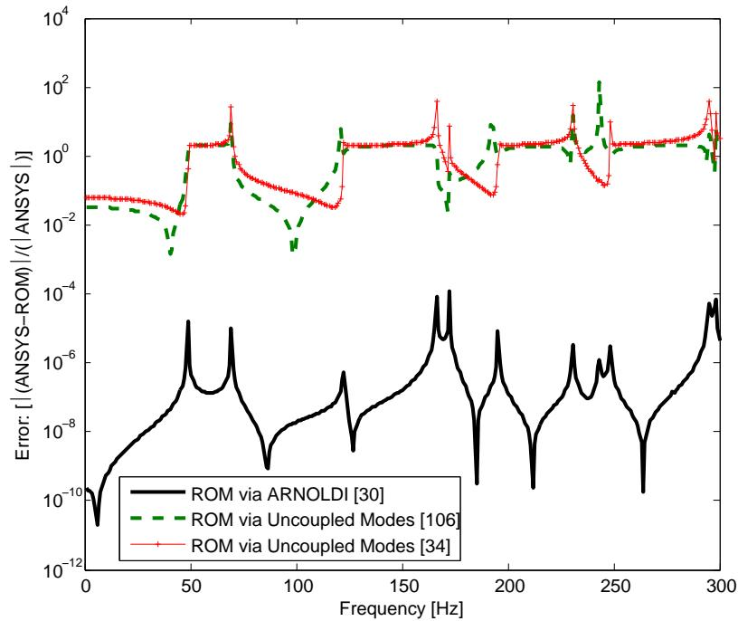
Figure 5.53.: A comparison of error quantities for driving point displacements for structural node at  $(0.25\text{m}, 1\text{m}, 0.65\text{m})$  obtained using Arnoldi projection, Uncoupled modes approach (Full) and Truncated uncoupled modal approach for  $\zeta=0$ .
