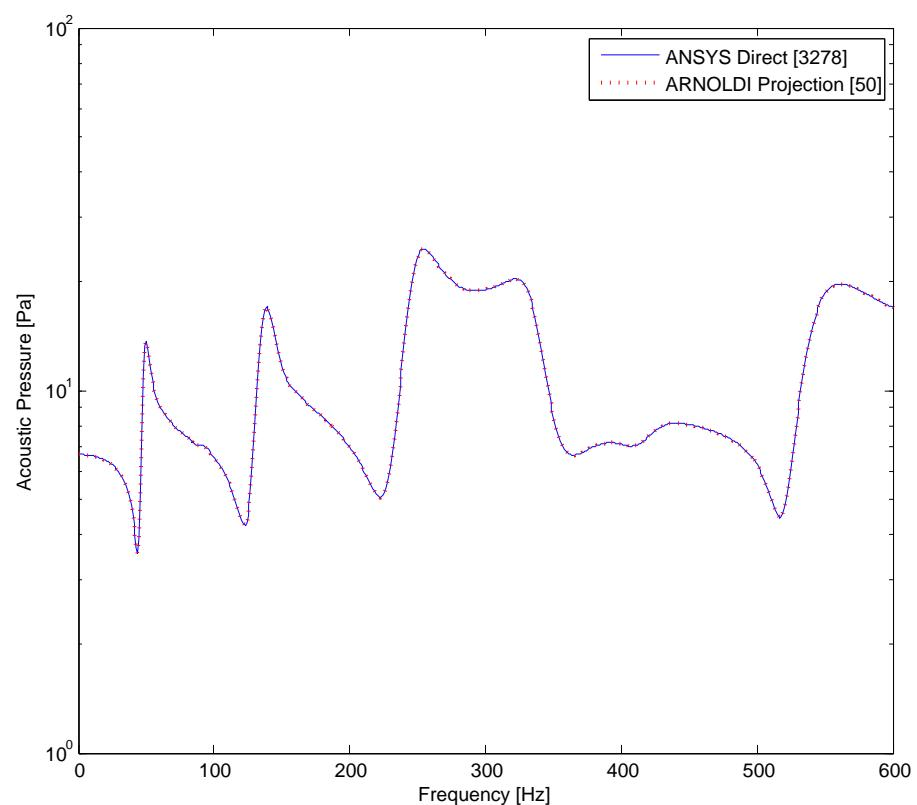
Figure 5.69.: Predicted Fluid Noise Transfer Function using direct and moment-matching Arnoldi (OSA) projection for fluid node at  $(0.135\text{m}, 0.07\text{m}, 0.175\text{m})$  for  $\zeta=0.05$ .
