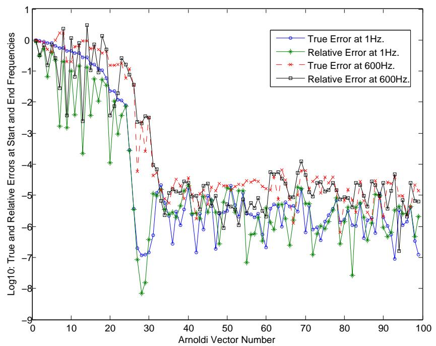
Figure 5.81.: Convergence pattern for moment-matching Arnoldi (TS-SOAR) projection at 1Hz and 600Hz for  $\beta_j^m=2.0E-05$ .
