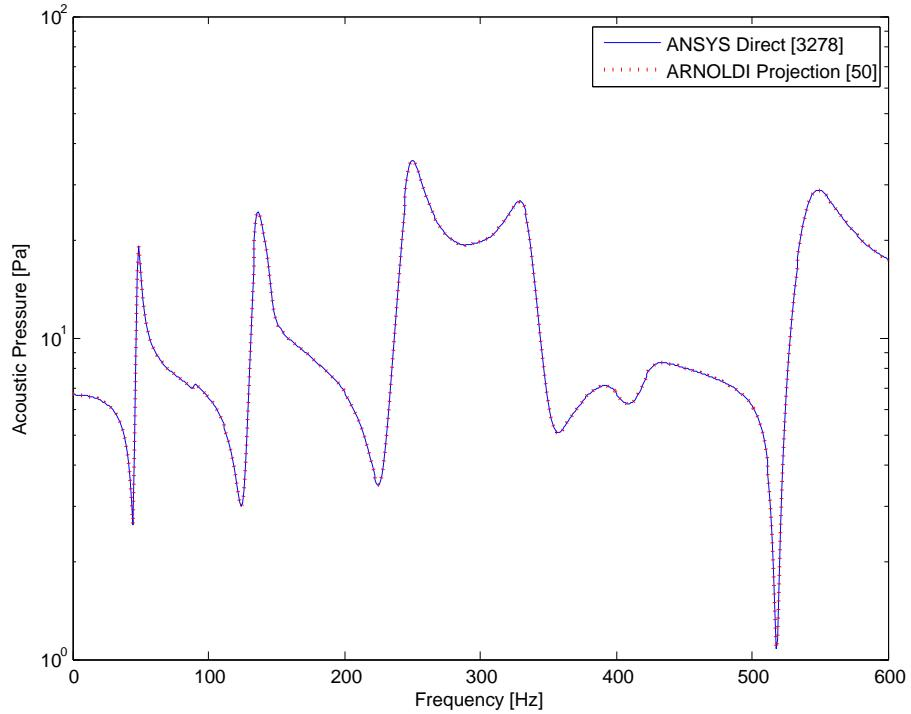
Figure 5.67.: Predicted Fluid Noise Transfer Function using direct and moment-matching Arnoldi (OSA) projection for fluid node at  $(0.135\text{m}, 0.07\text{m}, 0.175\text{m})$  for  $\zeta=0.03$ .
