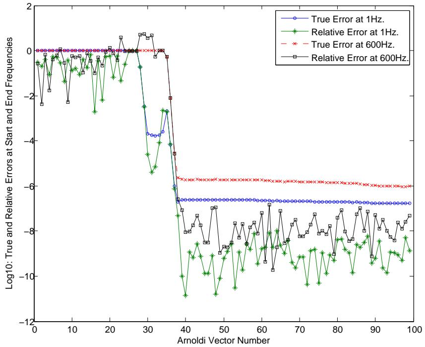
Figure 5.72.: Convergence pattern for moment-matching Arnoldi (OSA) projection at  $\omega=1\text{Hz}$  and  $\omega=600\text{Hz}$  for  $\zeta=0.10$ .
