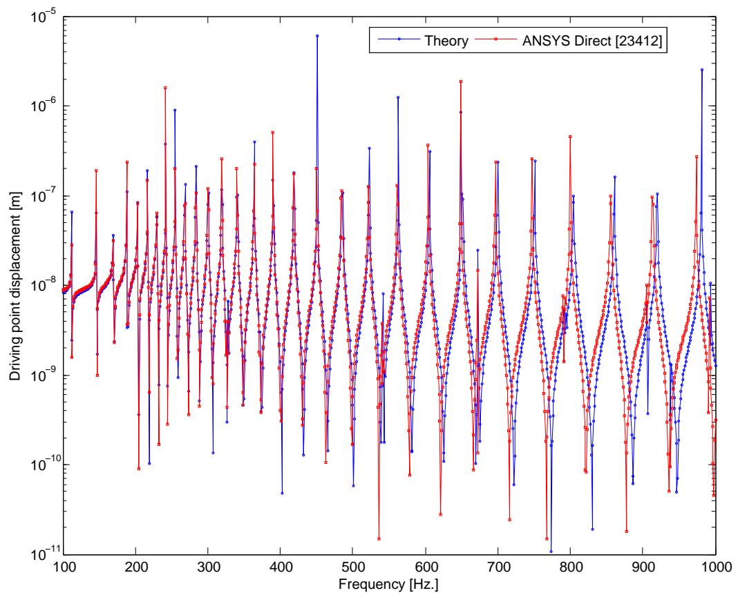
Figure 5.7.: A comparison of ANSYS direct inversion and analytical solution (Stepanishen and Cox 2000; ABAQUS 2005) for the prediction of driving point displacement.
