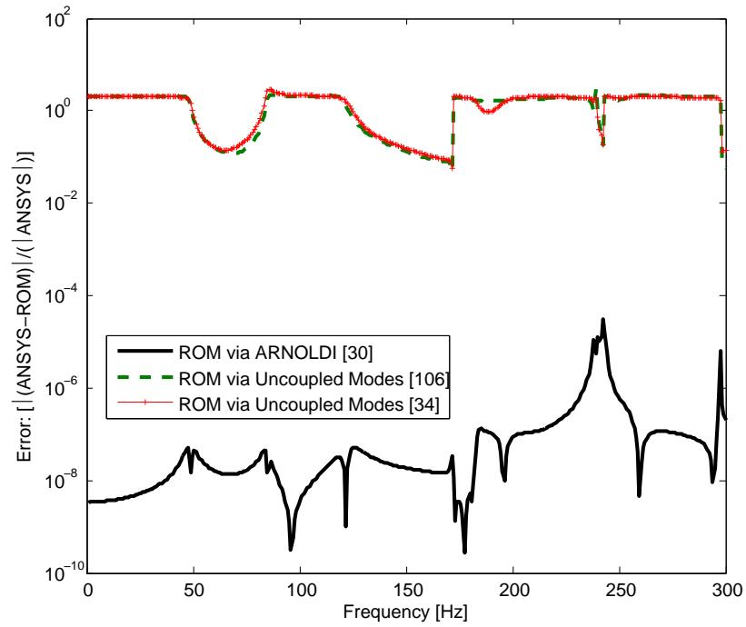
Figure 5.55.: A comparison of error quantities for noise transfer function for fluid node at  $(0.75\text{m}, 0.75\text{m}, 0.25\text{m})$  obtained using Arnoldi projection, Uncoupled modes approach (Full) and Truncated uncoupled modal approach for  $\zeta=0.03$ .
