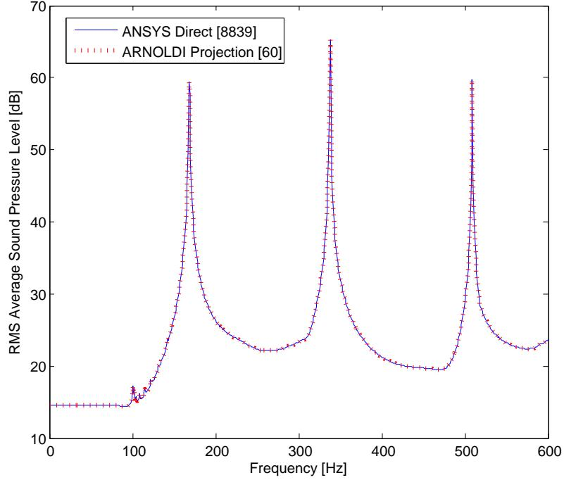
Figure 5.107.: Predicted RMS Averaged Fluid Noise Transfer Function using direct and moment-matching Arnoldi projection utilizing 21 fluid pressure outputs along the central axis of the clamped cylinder model [TC4<sub>CD2</sub>] with  $\zeta=0.10$ .
