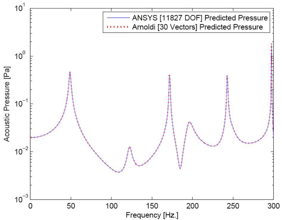
Figure 5.39.: ANSYS and moment matching Arnoldi projection predicted fluid pressure at  $(0.35\text{m}, 0.65\text{m}, 0.30\text{m})$  for  $\zeta=0.02$ .
