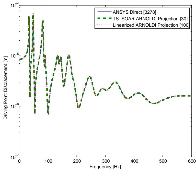
Figure 5.76.: Predicted Driving Point Displacement Transfer Function (Receptance) using direct and moment-matching Linearized Arnoldi and TS-SOAR projection for structural node at (0.039m,0.14m,0.078m) for  $\beta_j^m=6.0\text{E-}05$ .
