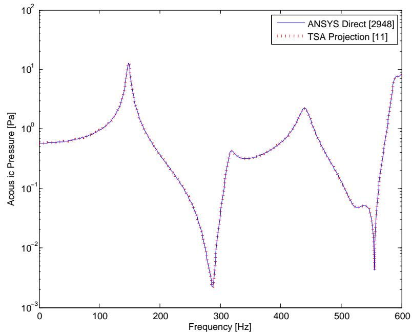
Figure 5.87.: Predicted Noise Transfer Function (NTF) using direct and moment-matching TSA projection for fluid node at (0.135m,0.07m,0.175m) for the air filled, clamped plate model.
