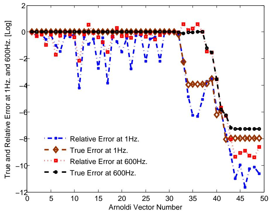
Figure 5.66.: Test Case No. 3: Convergence pattern for Arnoldi vectors at 1Hz and 600Hz.
