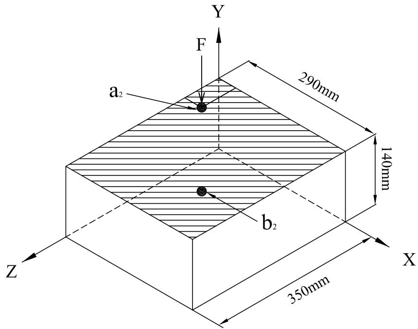
Figure 5.57.: Test Case No. 3: Plate backed rectangular cavity (water filled) system.
