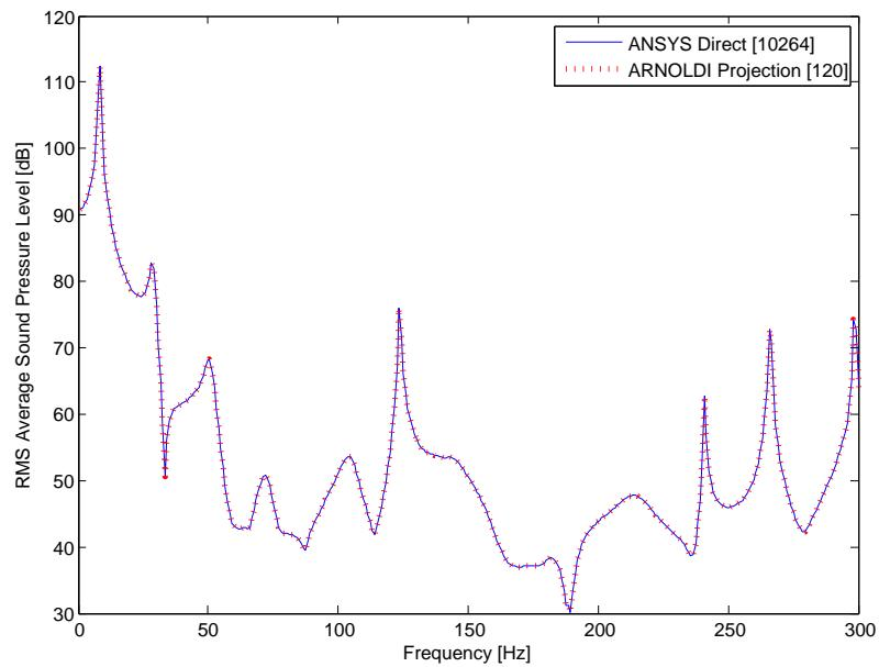
Figure 5.124.: Test Case No. 5: RMS averaged Noise Transfer Function for fluid nodes at  $(0.766\text{m}, 0.452\text{m}, 0.249\text{m})$ ,  $(0.33\text{m}, 0.38\text{m}, 0.24\text{m})$ ,  $(0.86\text{m}, 0.45\text{m}, 0.29\text{m})$ .
