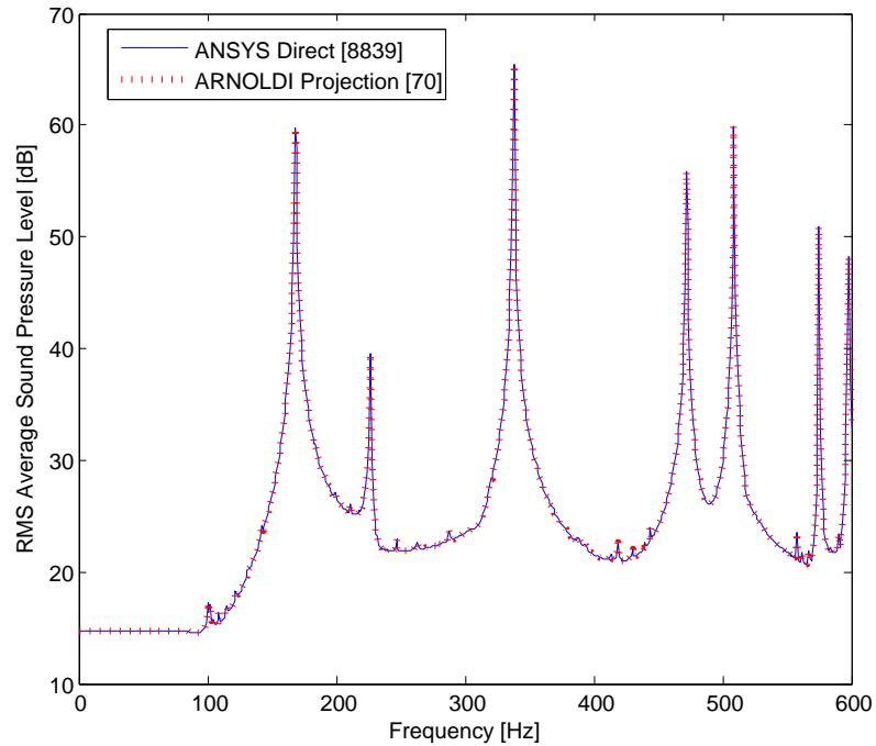
Figure 5.101.: Predicted RMS Averaged Fluid Noise Transfer Function using direct and moment-matching Arnoldi projection utilizing 21 fluid pressure outputs along the central axis of the clamped cylinder model [ $TC4_{CL}$ ].
