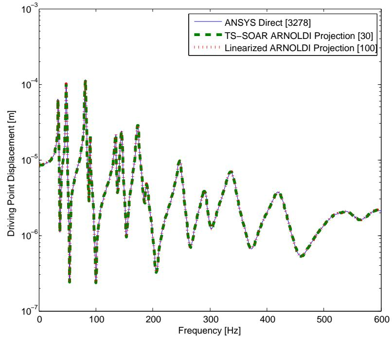
Figure 5.74.: Predicted Driving Point Displacement Transfer Function (Receptance) using direct and moment-matching Linearized Arnoldi and TS-SOAR projection for structural node at (0.039m,0.14m,0.078m) for  $\beta_j^m=2.0E-05$ .
