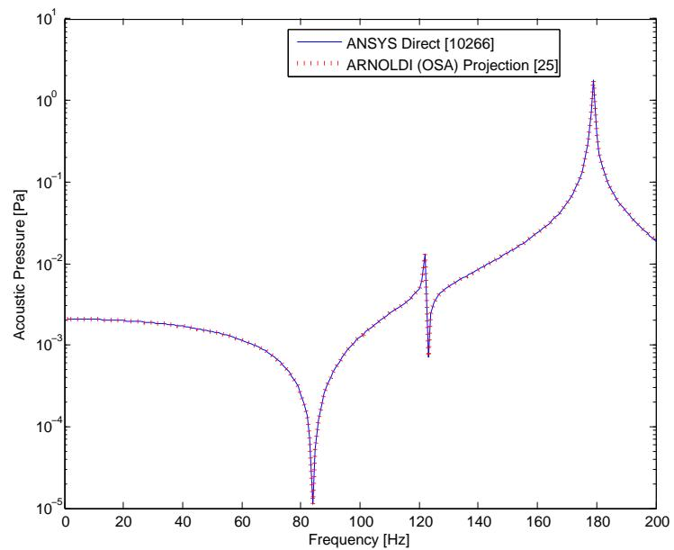
Figure D.2.: A comparison of noise transfer function obtained by ANSYS direct and One-sided Arnoldi (OSA) projection for optimized 8 layer stacking sequence (with material E-Glass Fiber composite).
