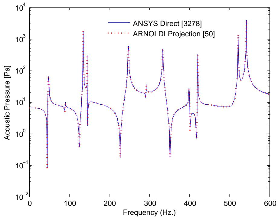
Figure 5.63.: Test Case No. 3: Predicted Fluid Noise Transfer Function (NTF) using direct and moment-matching Arnoldi projection for structural node at (0.135m,0.07m,0.175m).
