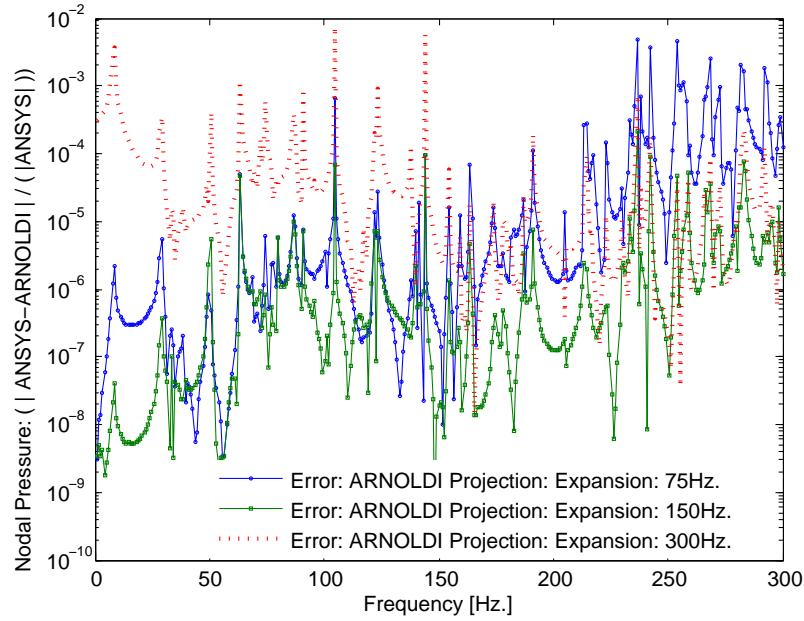
Figure 5.121.: Test Case No. 5: Noise Transfer Function error plot for fluid node at  $(0.33\text{m}, 0.38\text{m}, 0.24\text{m})$  for  $f_{exp}^1=75\text{Hz}$ ;  $f_{exp}^2=150\text{Hz}$ ;  $f_{exp}^3=300\text{Hz}$ .
