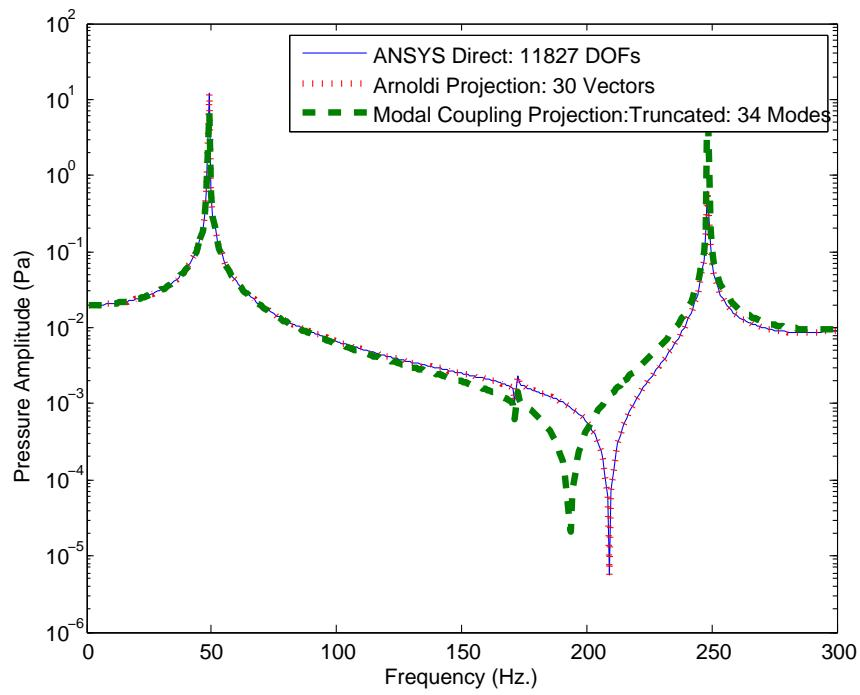
Figure 5.48.: ANSYS direct and truncated uncoupled modes (fluid+structure) projection predicted noise transfer functions for fluid node at (0.5m,0.5m,0.5m) for  $\zeta=0$ .
