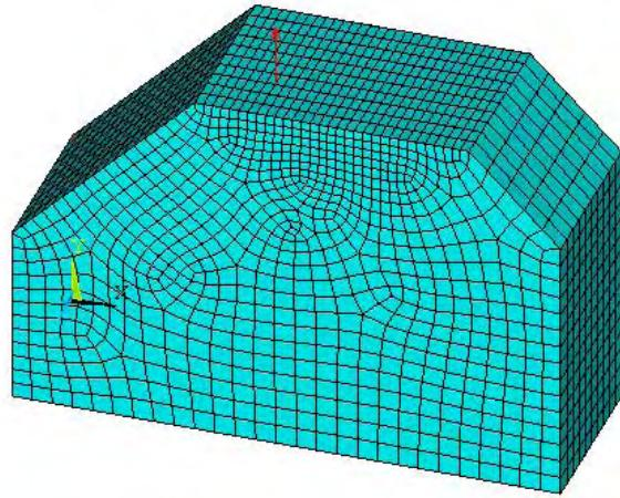
Figure 6.4.: Coupled Structural-Acoustic model for vibro-acoustic optimization.
