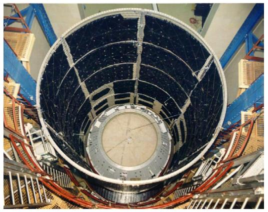
Figure 1.4.: Noise control of fairing by using acoustic heavy blankets.
