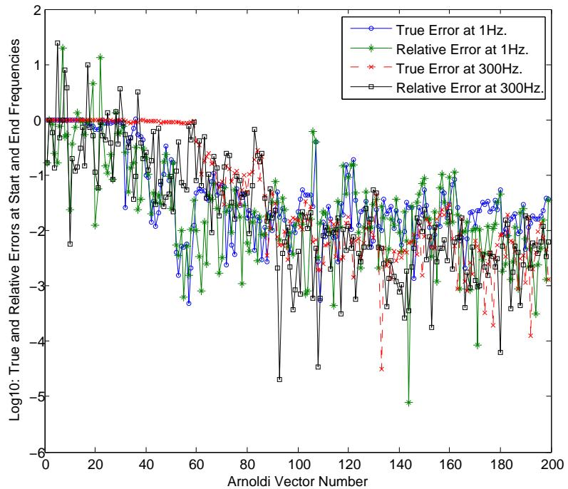
Figure 5.135.: Test Case No. 6: Convergence plot for Arnoldi vectors at approximately 1Hz and 300Hz for Terostat adhesive with constant acoustic damping [TC6<sub>Tac</sub>].
