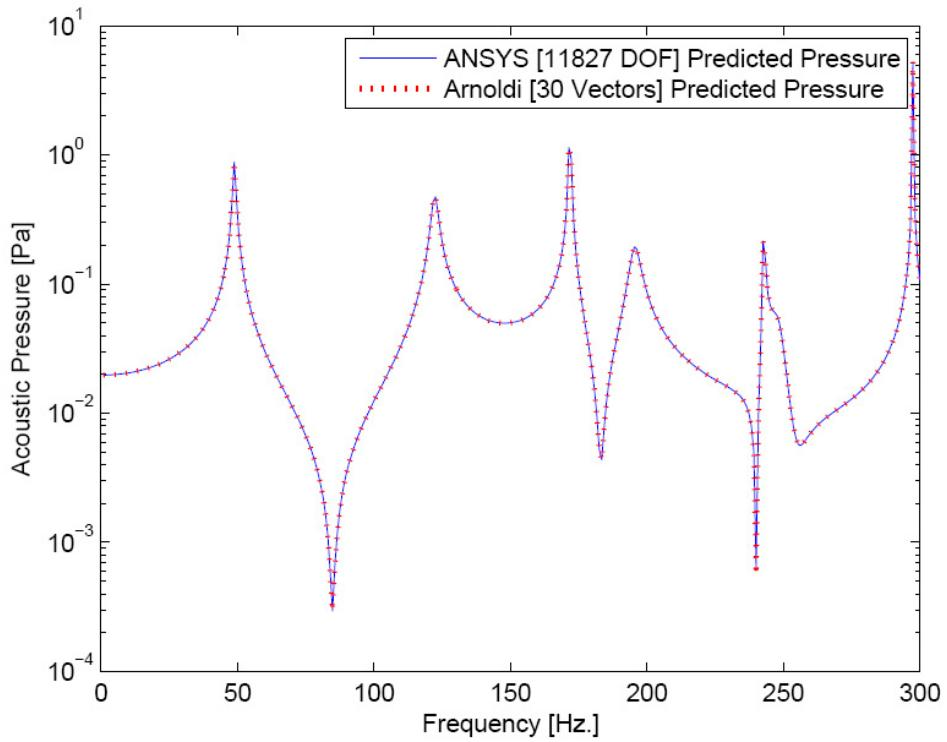
Figure 5.38.: ANSYS and moment matching Arnoldi projection predicted fluid pressure at  $(0.75\text{m}, 0.75\text{m}, 0.25\text{m})$  for  $\zeta=0.01$ .
