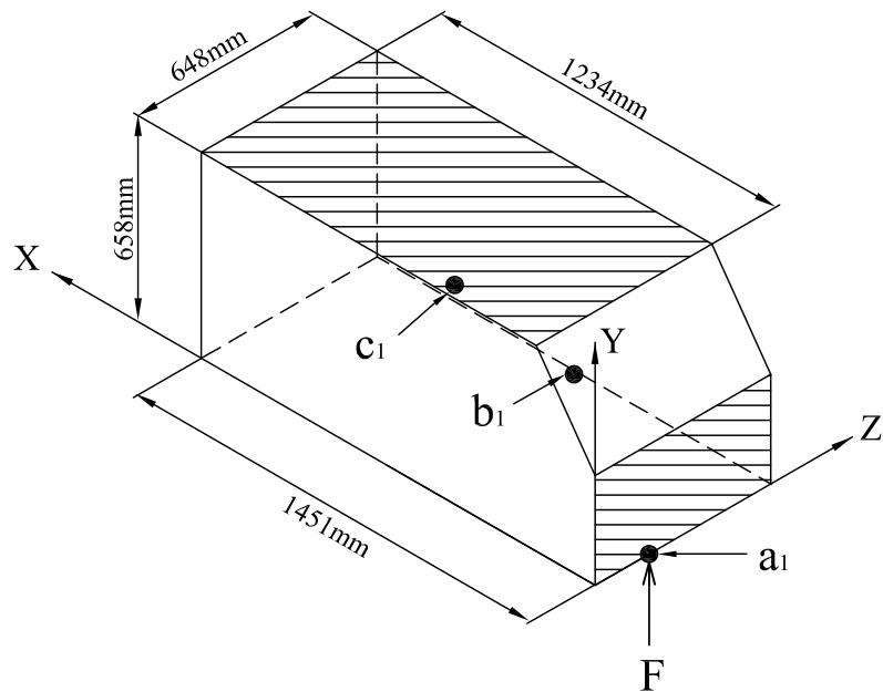
Figure 5.116.: Test Case No. 5: Beam-Plate model structure. Excitation location:  $a_1 = (0, 0, 0.2m)$ ; Measurement location(s):  $b_1 = (0.332m, 0.38m, 0.249m)$ ,  $c_1 = (0.766m, 0.452m, 0.249m)$ .
