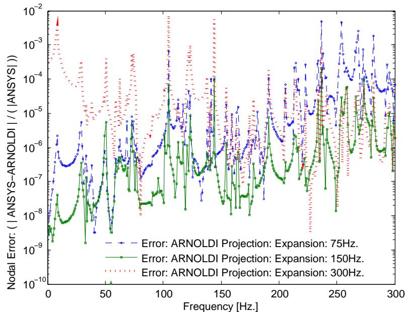
Figure 5.122.: Test Case No. 5: Noise Transfer Function error plot for fluid node at  $(0.76\text{m}, 0.45\text{m}, 0.24\text{m})$  for  $f_{exp}^1=75\text{Hz}$ ;  $f_{exp}^2=150\text{Hz}$ ;  $f_{exp}^3=300\text{Hz}$ .
