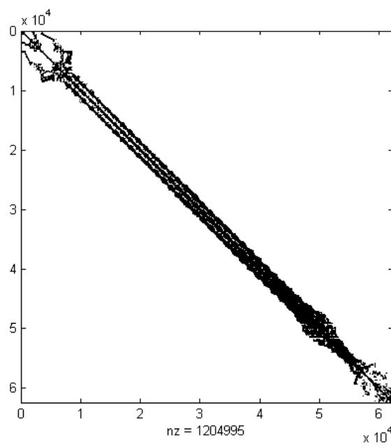
Figure C.1.: Test Case No. 6: Sparsity plot for coupled Stiffness Matrix.
