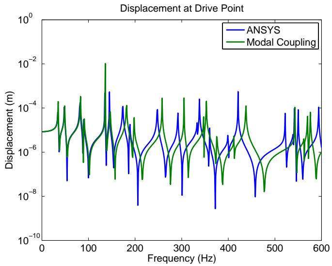
Figure B.1.: Test Case No. 3: Predicted driving point structural displacement transfer function (receptance) using direct and uncoupled modal coupling projection.
