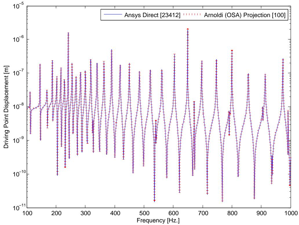
Figure 5.8.: A comparison of ANSYS direct inversion and One-Sided Arnoldi (OSA) prediction of driving point displacement.
