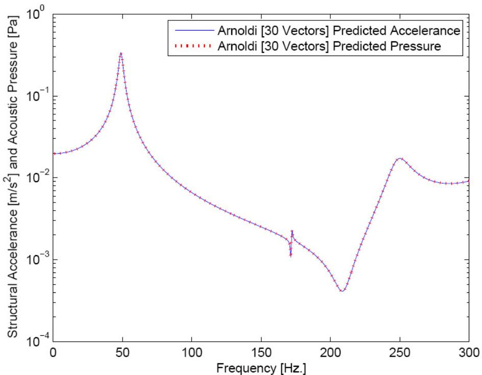
Figure 5.37.: Moment matching Arnoldi projection predicted vibro-acoustic reciprocity transfer functions for structural node at  $(0.25\text{m}, 1.0\text{m}, 0.65\text{m})$  and fluid node at  $(0.5\text{m}, 0.5\text{m}, 0.5\text{m})$  for  $\zeta=0.03$ .
