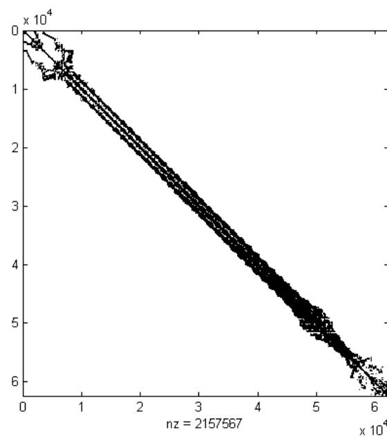
Figure C.2.: Test Case No. 6: Sparsity plot for coupled Mass Matrix.
