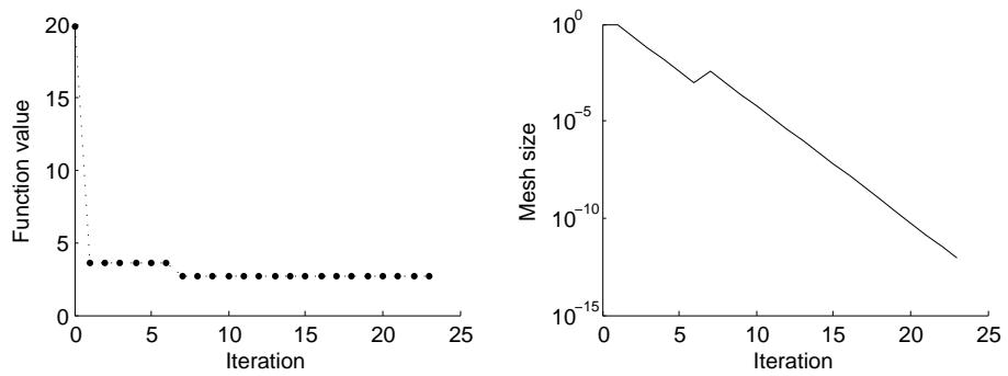
Figure 6.7.: Change in RMS objective function value (*left*) and mesh size (*right*) during optimization with initial 150 samples from LHS and starting stacking sequence  $[0/0]_{sym}$
