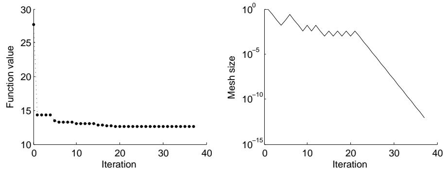
Figure 6.14.: Change in RMS objective function value (*left*) and mesh size (*right*) during optimization with initial 150 samples from LHS and with a starting stacking sequence  $[0/0/0/0]_{sym}$  for PP-Glass fiber composite.
