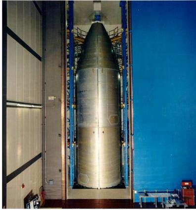
Figure 1.3.: Launch vehicle fairing structure (NASA 1996).
