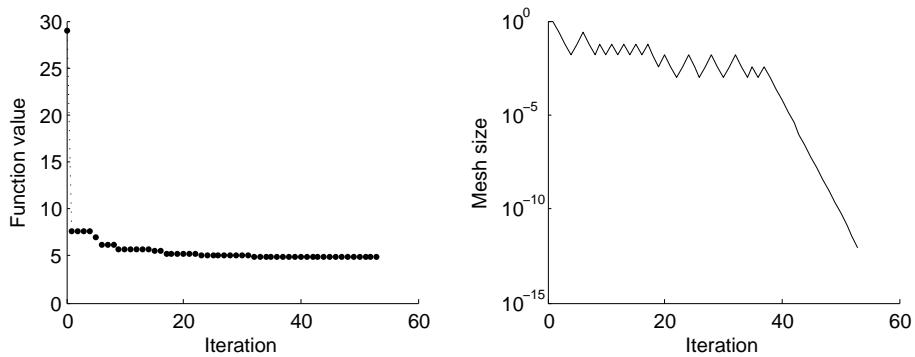
Figure 6.9.: Change in RMS objective function value (*left*) and mesh size (*right*) during optimization with initial 150 samples from LHS and with a starting stacking sequence  $[0/0/0/0]_{sym}$  for E-Glass fiber composite.
