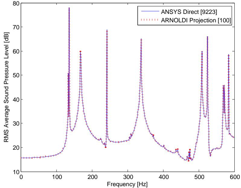
Figure 5.98.: Predicted RMS Averaged Fluid Noise Transfer Function using direct and moment-matching Arnoldi projection utilizing 21 fluid pressure outputs along the central axis of the undamped free-free cylinder [TC4<sub>FF</sub>].
