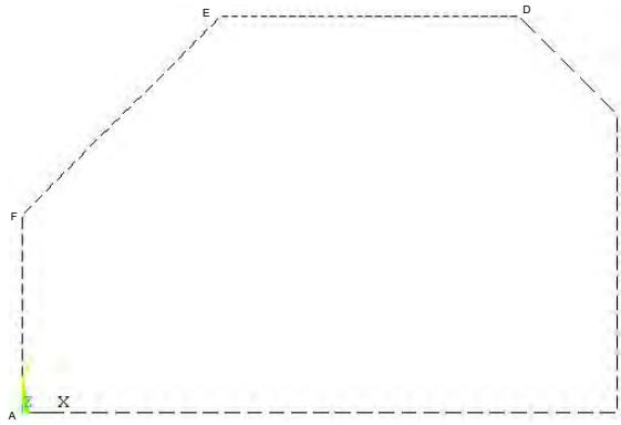
Figure 6.3.: 2-D cross section of the rectangular prism considered for the coupled structural acoustic optimization.
