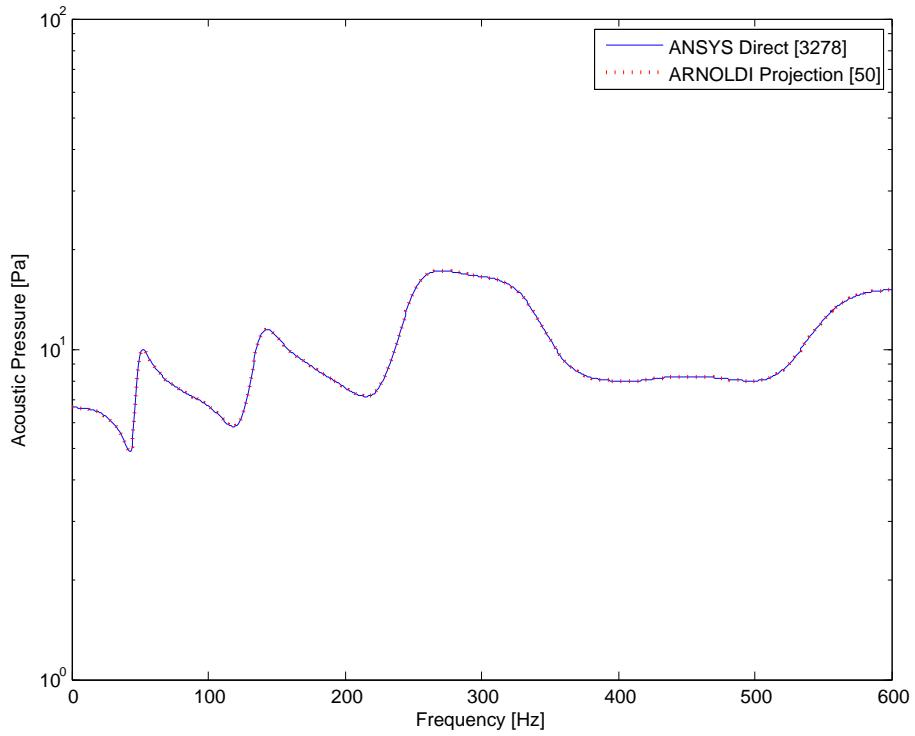
Figure 5.71.: Predicted Fluid Noise Transfer Function using direct and moment-matching Arnoldi (OSA) projection for fluid node at  $(0.135\text{m}, 0.07\text{m}, 0.175\text{m})$  for  $\zeta=0.10$ .
