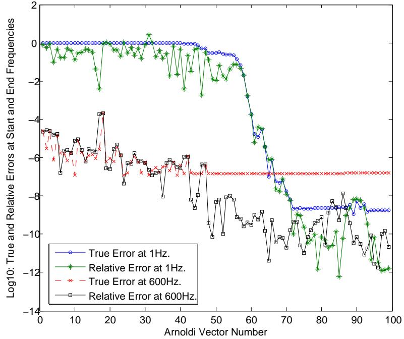
Figure 5.103.: Convergence pattern for 21 fluid pressure outputs [TC4<sub>CL</sub>].
