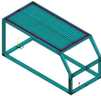
Figure 5.127.: Test Case No. 6: Structural model with adhesive bond (pink elements).
