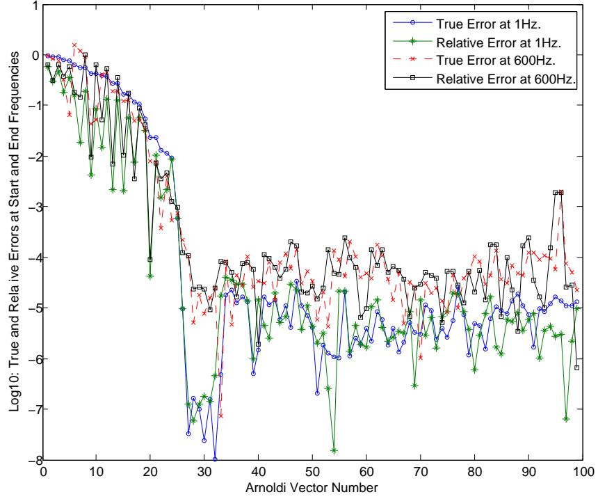
Figure 5.83.: Convergence pattern for moment-matching Arnoldi (TS-SOAR) projection at 1Hz and 600Hz for  $\beta_j^m=6.0\text{E-}05$ .
