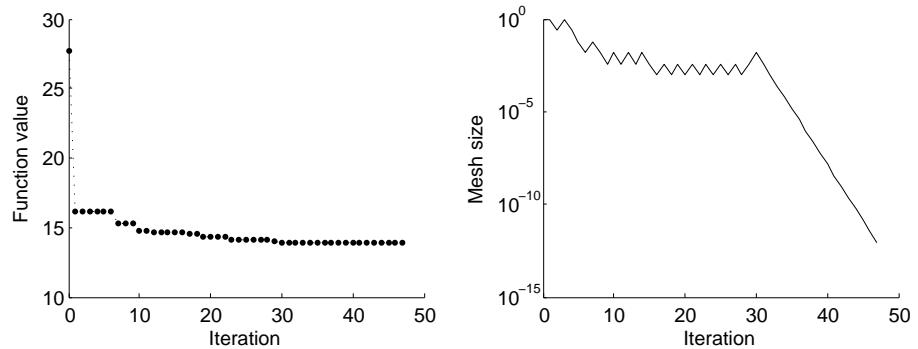
Figure 6.13.: Change in RMS objective function value (*left*) and mesh size (*right*) during optimization with initial 100 samples from LHS and with a starting stacking sequence  $[0/0/0/0]_{sym}$  for PP-Glass fiber composite.
