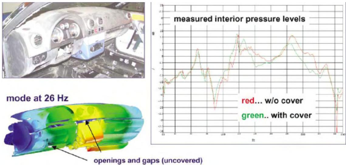
Figure 2.3.: Effects of gaps and openings on interior SPL (Priebsch et al. 2001).
