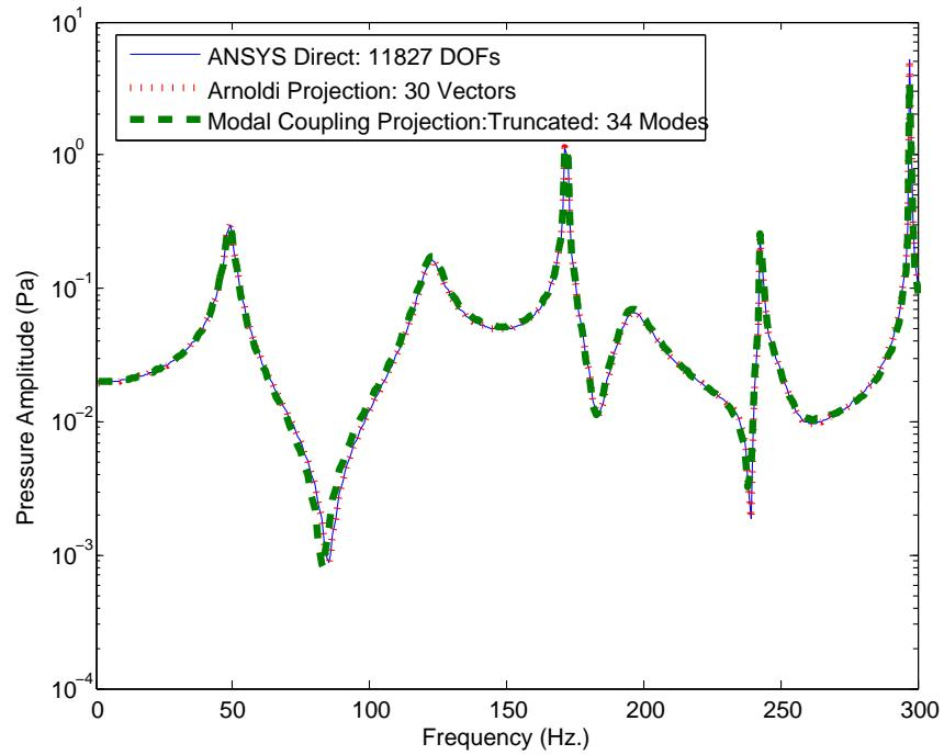
Figure 5.49.: ANSYS direct and truncated uncoupled modes (fluid+structure) projection predicted noise transfer functions for fluid node at (0.75m,0.75m,0.25m) for  $\zeta=0.03$ .
