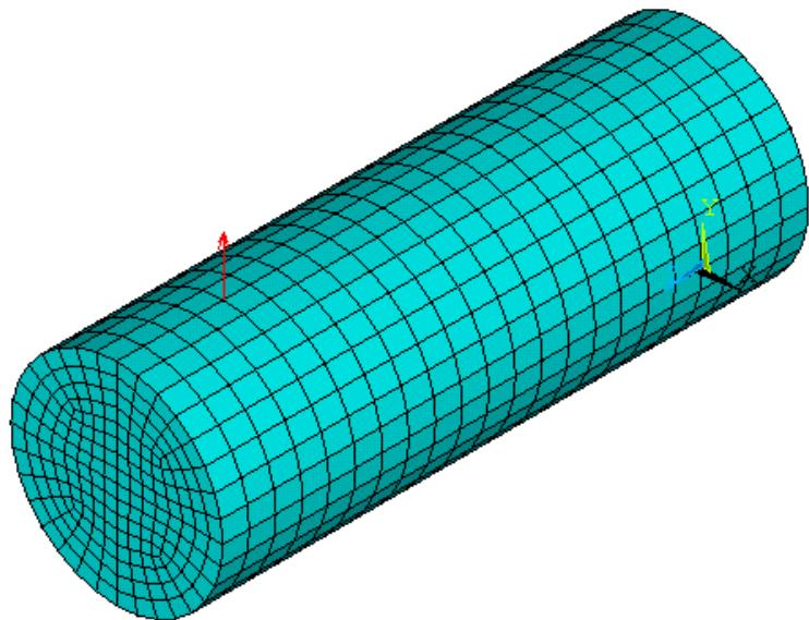
Figure 5.92.: Test Case No. 4: Free-Free Cylindrical cavity (air filled) system: Fully Coupled FE model.
