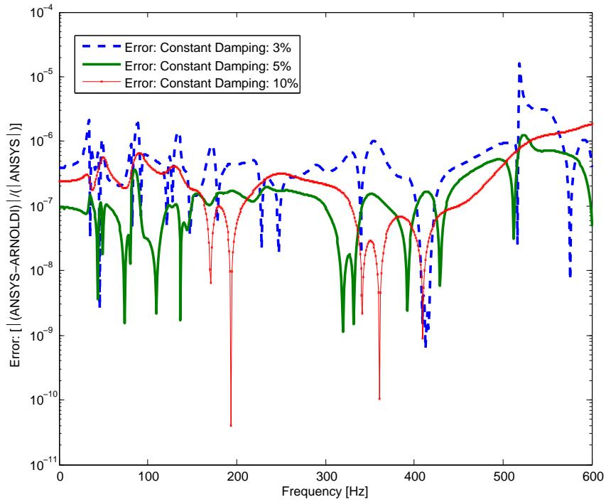
Figure 5.73.: Error plot for fluid grid point at  $(0.135\text{m}, 0.07\text{m}, 0.175\text{m})$  for damping values:  $\zeta=0.03$ ,  $\zeta=0.05$ ,  $\zeta=0.10$ .
