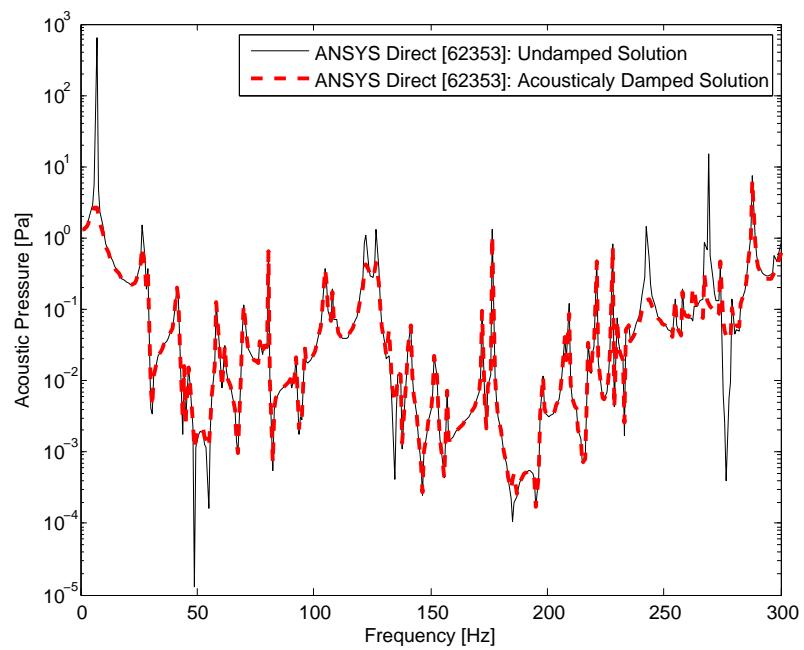
Figure C.6.: Test Case No. 6: A comparison of direct inversion predicted noise transfer at fluid node (0.9m,0.5m,0.08m) for undamped and constant acoustically damped model [TC6<sub>Tac</sub>].
