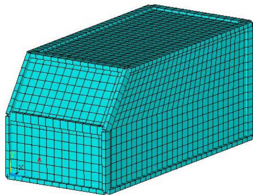
Figure 5.118.: Test Case No. 5: Fully coupled structural-acoustic FE Model.
