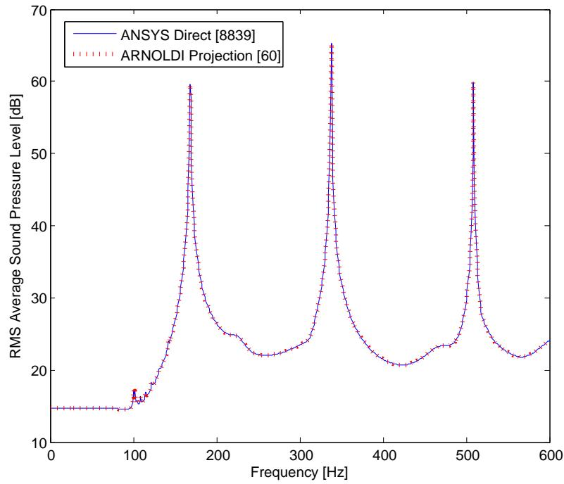
Figure 5.104.: Predicted RMS Averaged Fluid Noise Transfer Function using direct and moment-matching Arnoldi projection utilizing 21 fluid pressure outputs along the central axis of the clamped cylinder model [TC4<sub>CD1</sub>] with  $\zeta=0.05$ .
