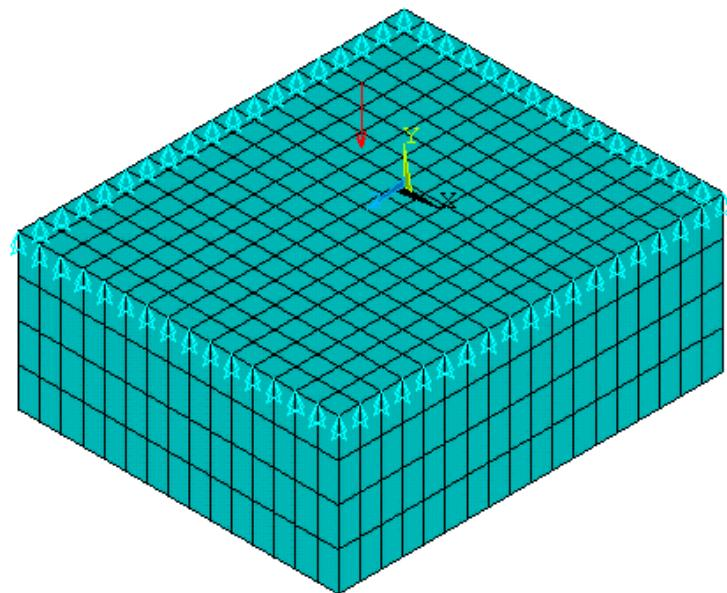
Figure 5.58.: Test Case No. 3: Fully Coupled FE model.
