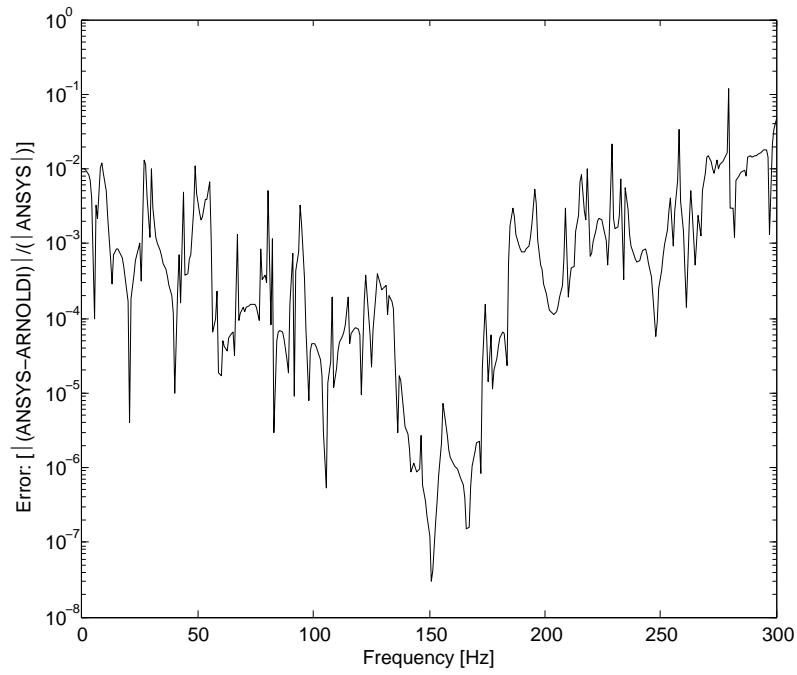
Figure 5.134.: Test Case No. 6: Noise Transfer Function error plot for structural acoustic model [TC6<sub>Tac</sub>].
