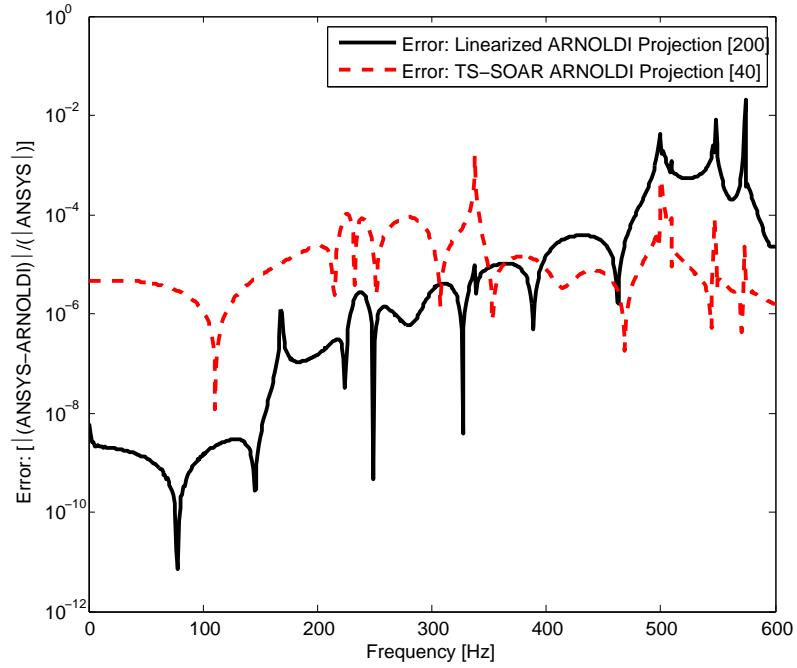
Figure 5.114.: Local Error quantities for ROMs generated via moment-matching Linearized OSA Arnoldi and TS-SOAR projection for fluid node at the center of the cylinder with  $\beta_j^m=7.0\text{E-}05$ .
