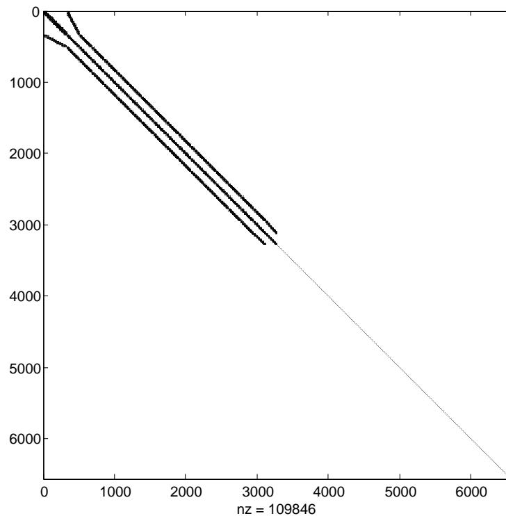
Figure 5.62.: Test Case No. 3: Equivalent Linearized System (Equation:4.70a)  $\mathbf{G}_{sa}$  sparsity plot for  $\beta_j^m=4.0\text{E-}05$  [TC3<sub>md</sub>].
