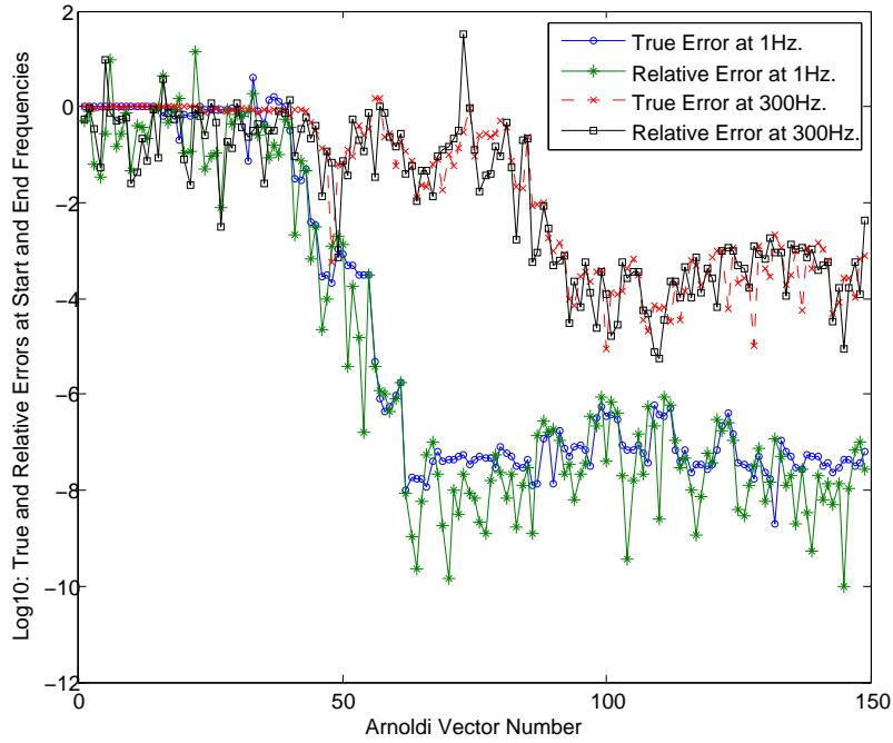
Figure 5.132.: Test Case No. 6: Convergence plot for Arnoldi vectors at approximately 1Hz and 300Hz for the coupled model with Terostat adhesive [TC6<sub>TT</sub>].
