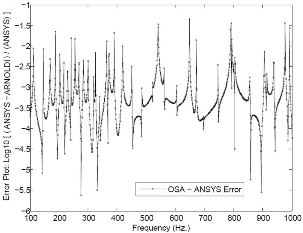
Figure 5.10.: Error Plot: ANSYS direct inversion and Arnoldi (OSA) predictions for fluid nodal pressure at the center of the acoustic domain.
