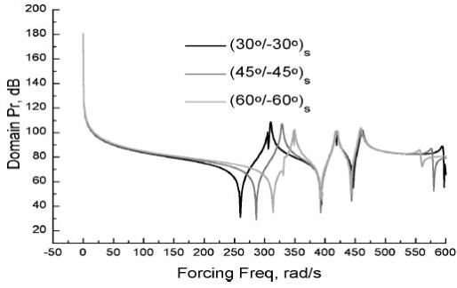
Figure 2.1.: Pressure variation with stack-ing sequence (Niyogi et al. 2000).
