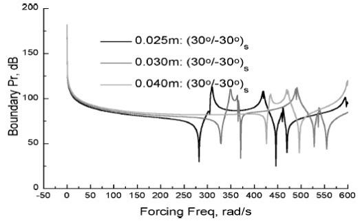
Figure 2.2.: Pressure variation with stack-ing sequence and wall thickness (Niyogi et al. 2000).
