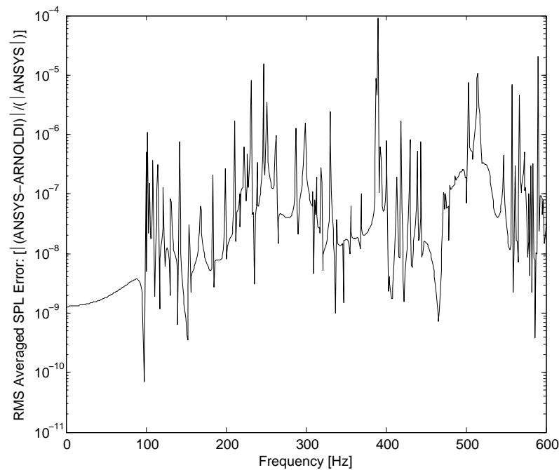
Figure 5.102.: Local RMS Averaged Error Plot utilizing 21 fluid pressure outputs [ $TC4_{CL}$ ].
