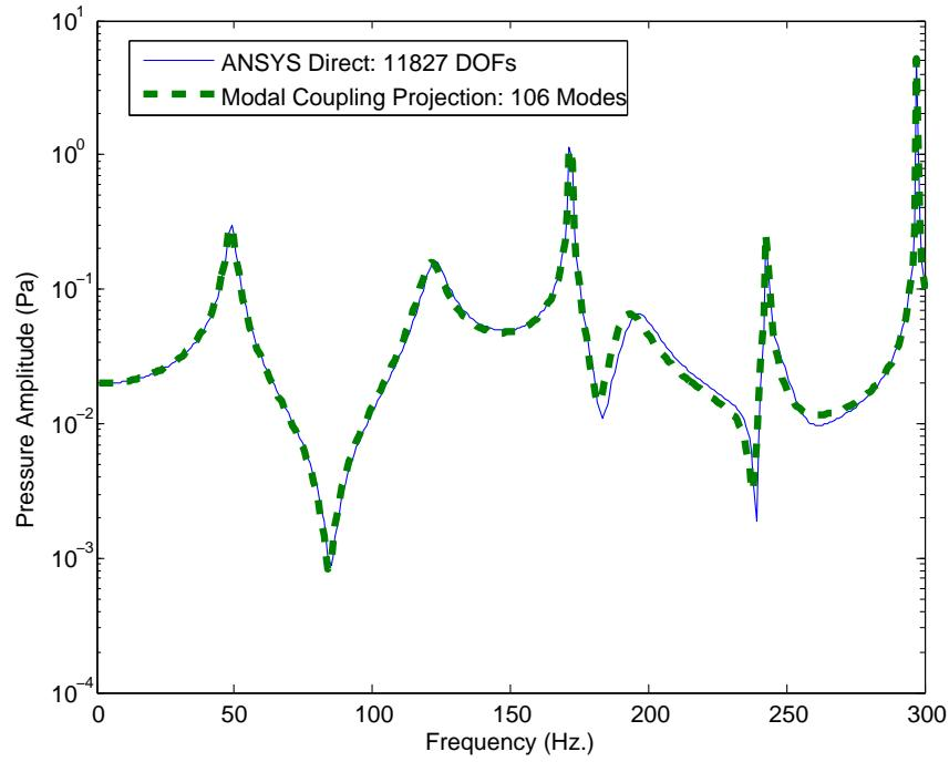
Figure 5.52.: ANSYS direct and uncoupled modes (fluid+structure) projection predicted noise transfer functions for fluid node at  $(0.75\text{m}, 0.75\text{m}, 0.25\text{m})$  for  $\zeta=0.03$ .
