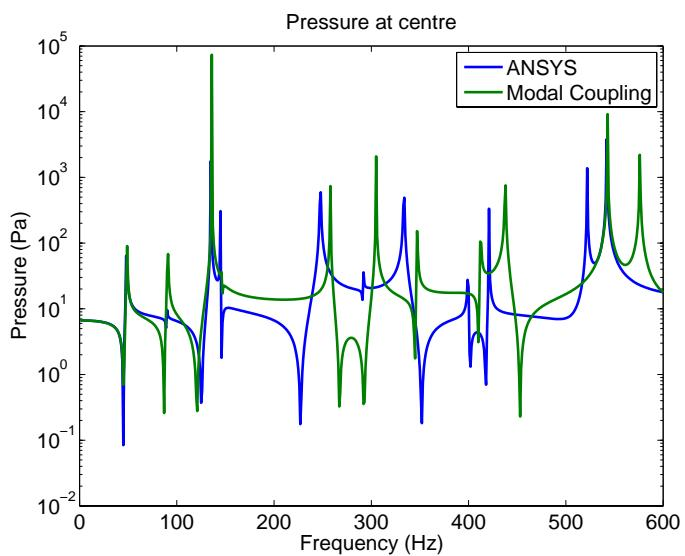
Figure B.2.: Test Case No. 3: Predicted Fluid Noise Transfer Function using direct and uncoupled modal coupling projection for fluid node at the center of the acoustic domain.
