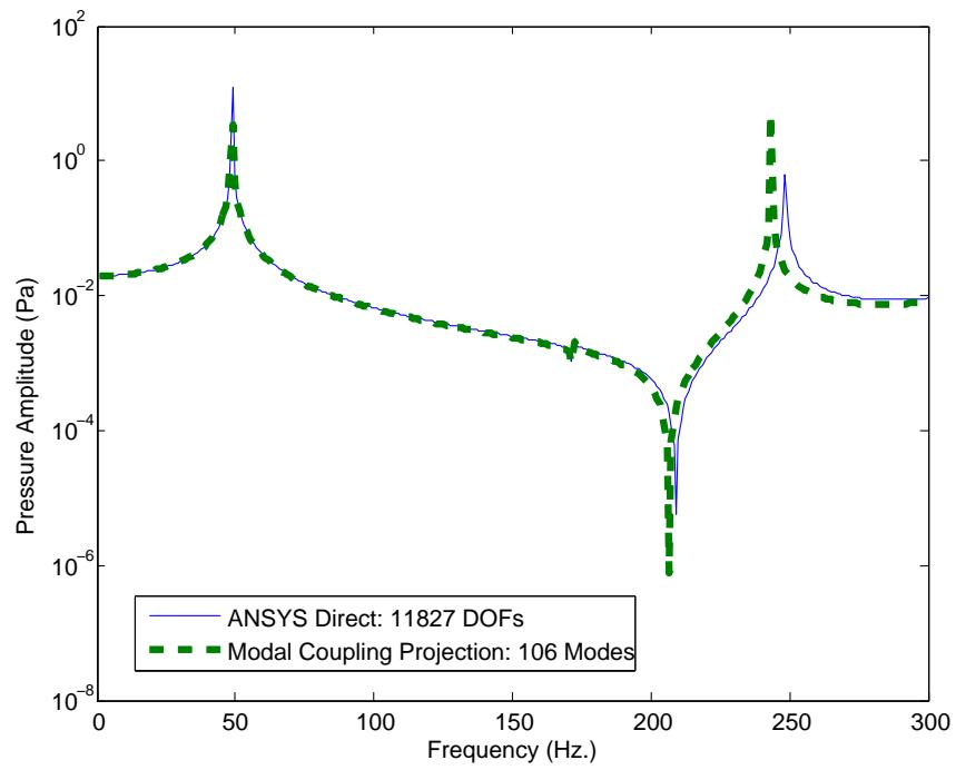
Figure 5.50.: ANSYS direct and uncoupled modes (fluid+structure) projection predicted noise transfer functions for fluid node at (0.5m,0.5m,0.5m) for  $\zeta=0$ .
