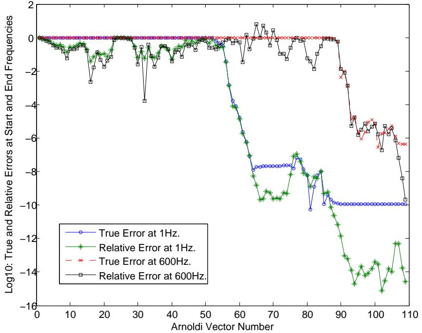
Figure 5.86.: Convergence pattern for moment-matching Linearized Arnoldi projection at 1Hz and 600Hz for  $\beta_j^m=6.0\text{E-}05$ .
