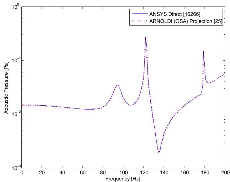
Figure D.1.: A comparison of noise transfer function obtained by ANSYS direct and One-sided Arnoldi (OSA) projection for optimized 4 layer stacking sequence.
