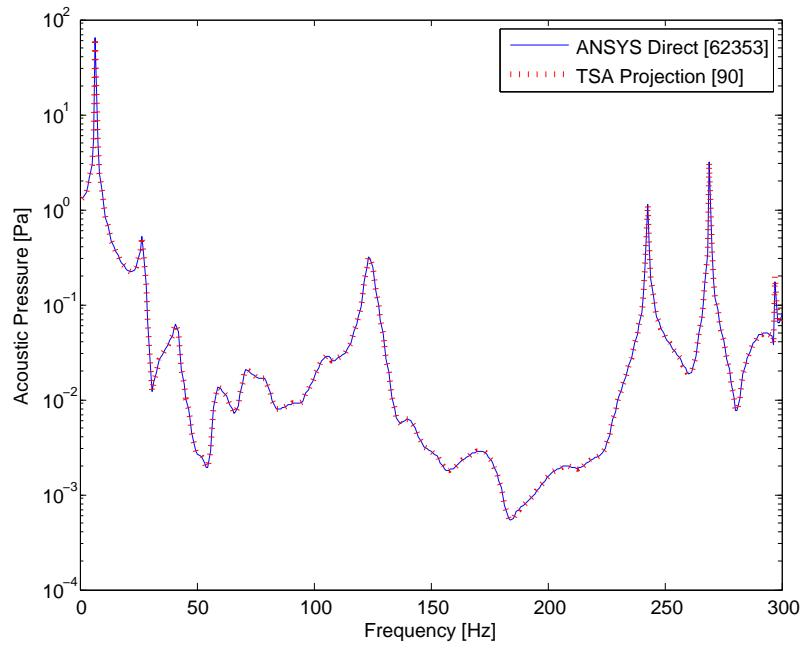
Figure C.5.: Test Case No. 6: ANSYS and TSA projection predicted Noise Transfer Function at fluid node (0.9m,0.5m,0.08m) for model TC6<sub>TT</sub>.
