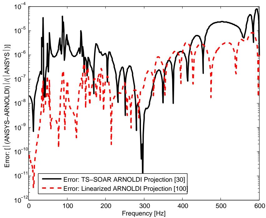
Figure 5.79.: Error plot for Predicted Driving Point Displacement Transfer Function (Receptance) at  $(0.039\text{m}, 0.14\text{m}, 0.078\text{m})$  for Linearized Arnoldi and TS-SOAR projections with damping value  $\beta_j^m = 4.0\text{E-}05$  [TC3<sub>md</sub>].
