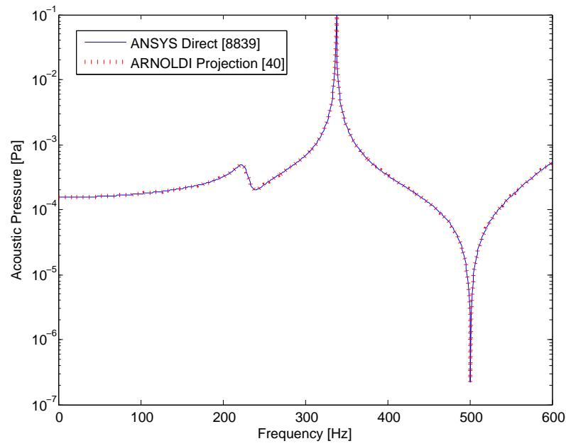
Figure 5.110.: Predicted Noise Transfer Function (NTF) using direct and moment-matching TS-SOAR projection for fluid node at the center of the cylindrical cavity model [TC4<sub>FD1</sub>] with  $\beta_j^m=5.0\text{E-}05$ .
