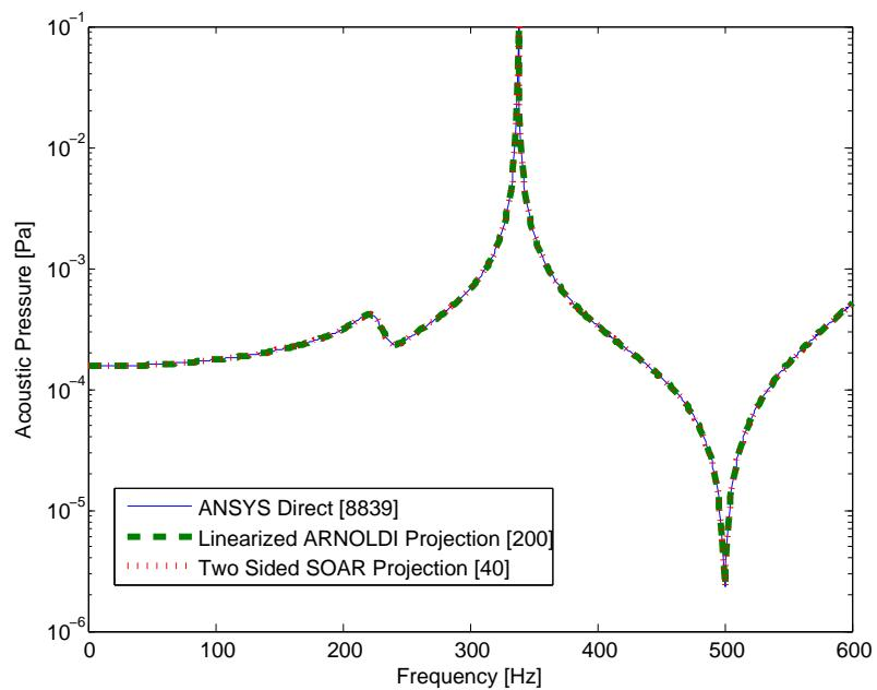
Figure 5.113.: Predicted Noise Transfer Function (NTF) using direct and moment-matching Linearized Arnoldi (OSA) and TS-SOAR projection for fluid node at the center of the cylindrical cavity model [TC4<sub>FD2</sub>] with  $\beta_j^m=7.0\text{E-}05$ .
