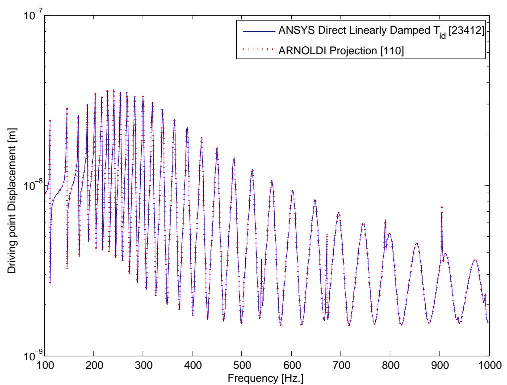
Figure 5.15.: A comparison between ANSYS direct inversion and Two-Sided Second order Arnoldi (TS-SOAR) predictions of driving point displacement for linearly damped,  $T_{ld}$  damping model.
