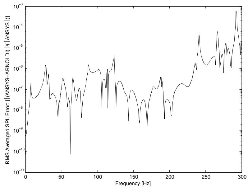
Figure 5.125.: Test Case No. 5: RMS averaged Noise Transfer Function error plot for fluid nodes at  $(0.766\text{m}, 0.452\text{m}, 0.249\text{m})$ ,  $(0.33\text{m}, 0.38\text{m}, 0.24\text{m})$ ,  $(0.86\text{m}, 0.45\text{m}, 0.29\text{m})$ .
