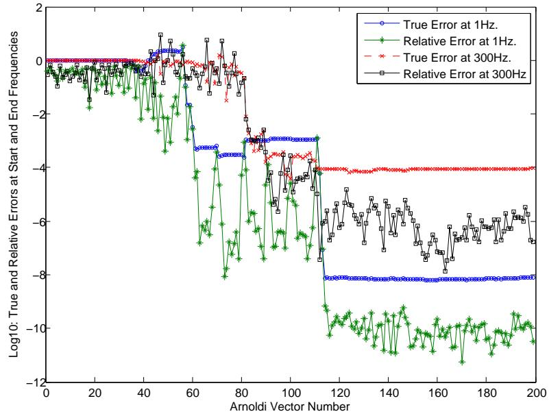
Figure 5.126.: Test Case No. 5: Convergence plot for Arnoldi vectors at approximately 1Hz and 300Hz.
