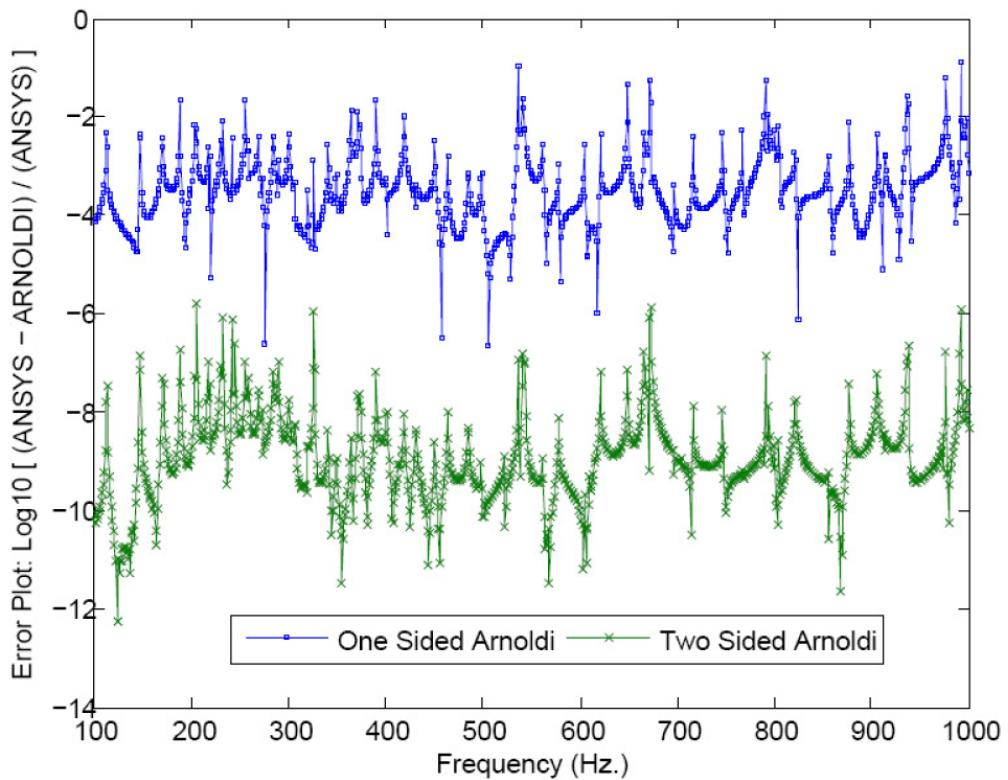
Figure 5.11.: Error Plot: ANSYS direct inversion, OSA and TSA predictions for structural driving point displacement.
