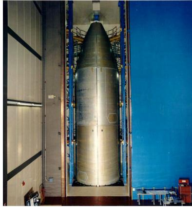
Figure 1.3.: Launch vehicle fairing structure (NASA 1996).
