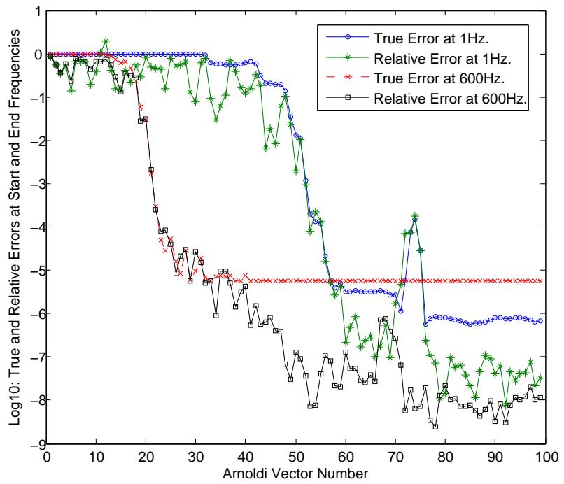
Figure 5.109.: Convergence pattern for moment-matching Arnoldi (OSA) projection at 1Hz and 600Hz for  $\zeta=0.10$ .
