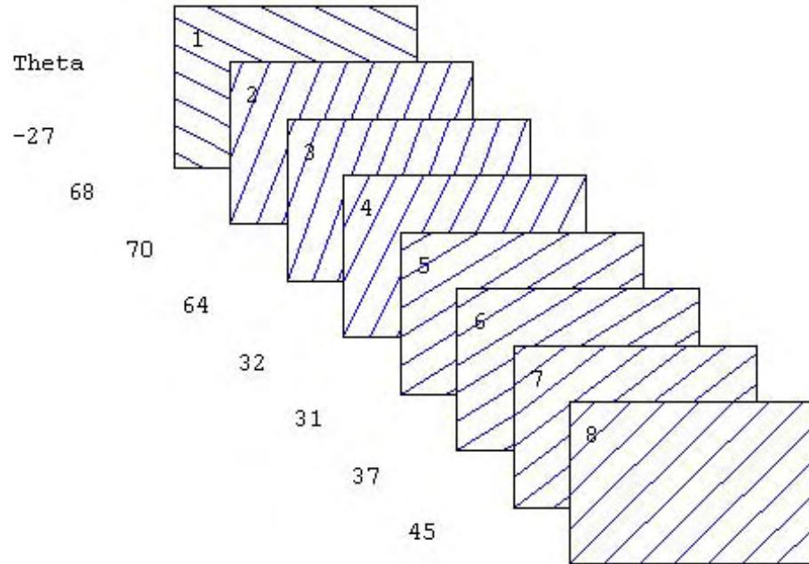
Figure 6.11.: Layer plot of optimum stacking sequence for E-Glass Fiber composite with wall thickness of 2.1mm with 8 layers.
